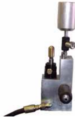
Figure 4. Insert the funnel with the needle valve into the manifold.
