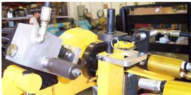
Figure 1. The photograph shows the autofeed system on the Guillotine saw. (The feed handle has been removed for autofeed operation.)
