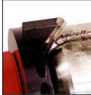
SDB 206 & 412 Insert Tooling System: Significantly reduces tooling costs. Tool holders for facing & beveling utilize replaceable double edge cutting inserts.
