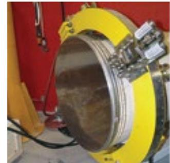
Simultaneously cuts and bevels out-of-round pipe
