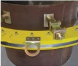
Standard with lifting rings for horizontal or vertical mounting.
