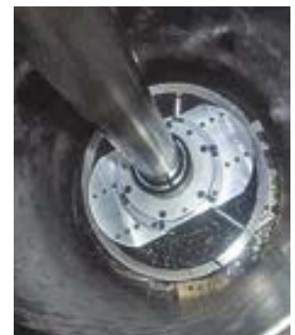
Internal cutting module lowered to cutting depth
