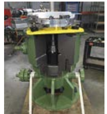
EICC Casing Cutter used for wellhead completion
