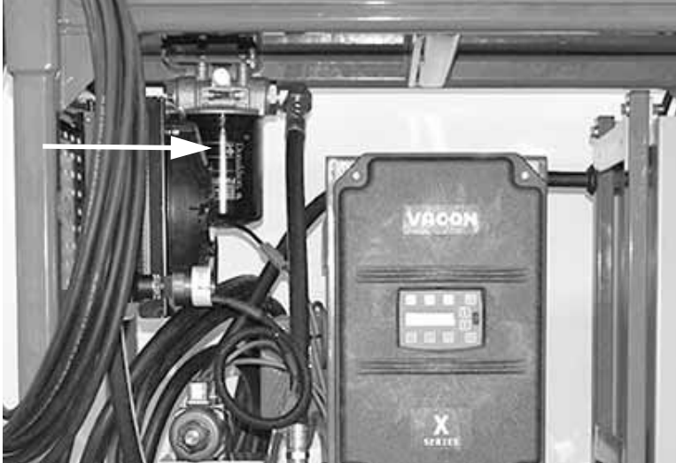
Figure 3-9. Replace the hydraulic oil filter every time you replace the hydraulic oil.
