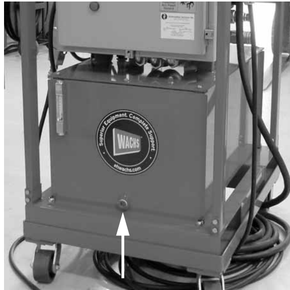
Figure 3-8. The hydraulic oil drain plug is at the bottom of the oil reservoir, on the front of the unit.
