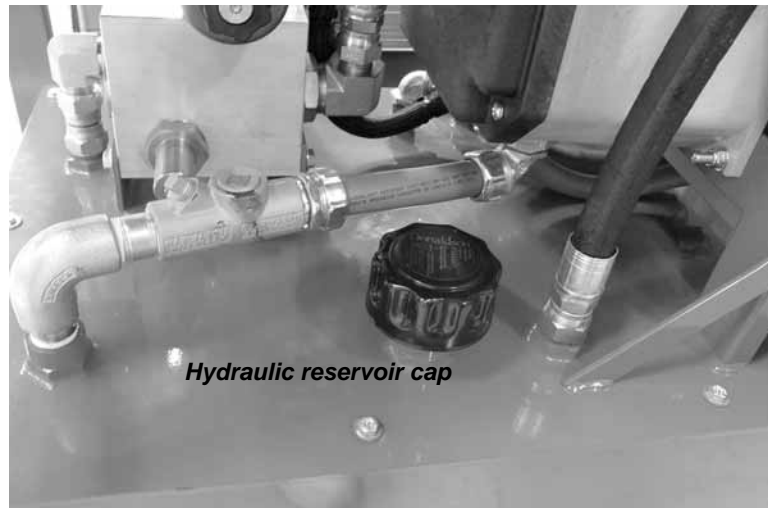
Figure 3-2. Remove the hydraulic reservoir cap and fill the reservoir with hydraulic oil (approximate capacity 30 gallons [114 l]).
