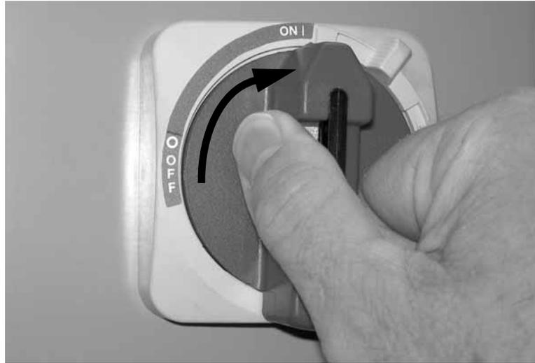
*Figure 1-11. Turn the power switch to the ON position.*
