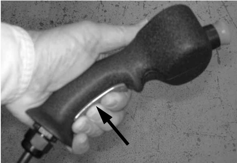
Figure 1-13. Squeeze the trigger to start the LCSF.
