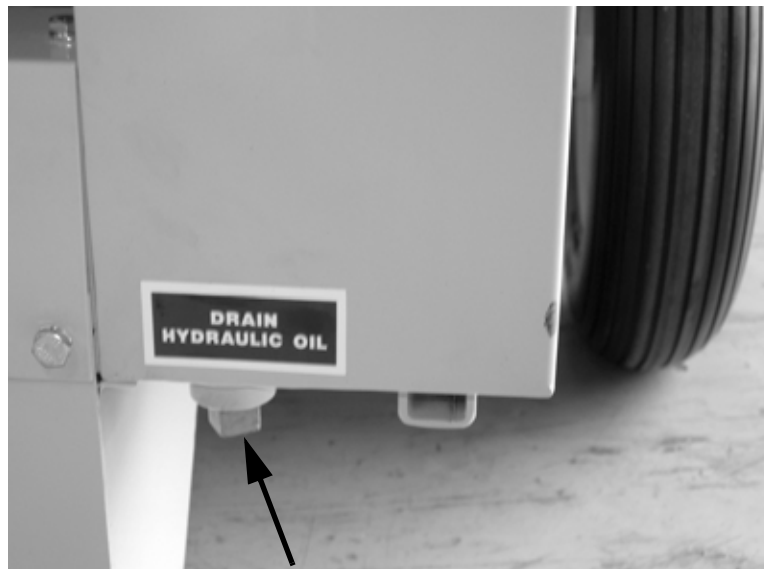
Figure 1-4. The hydraulic tank drain plug is at the bottom of the front panel.
