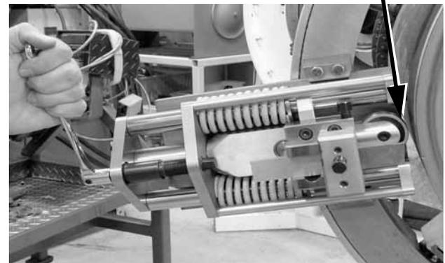
**WARNING:** Do not loosen the mounting block screws or try to remove the slides when the tracking wheels are under spring pressure against the pipe. The spring pressure will “pop” the slide away from the pipe. Serious injury or damage to the equipment can result.
