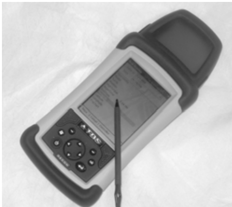
Figure 1. The Vitals controller with its pen stylus. The optional GPS receiver is located under the top “cap”.
