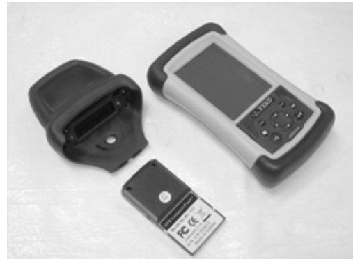
Figure 4. The photo shows the GPS receiver card and the extended cap that is provided with it.
