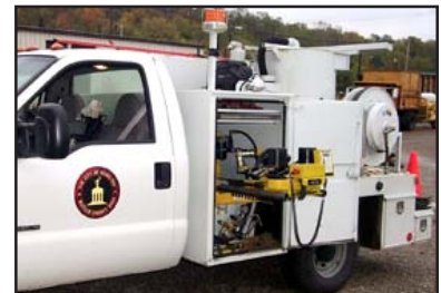
TM-7 valve operator with vertical tank Trav-L-Vac 300.
