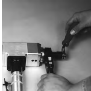
2. Remove draw bar using the clamp ratchet.
