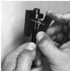
3. Slide the clamp leg set up the draw bar and slip leg set over draw bar head slot.
