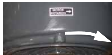
Motor should turn clockwise
