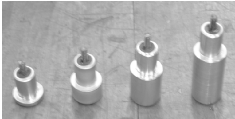
Figure 3-7. The four shorter clamping legs are used with the smaller cutting machine for the four smaller casing diameters.
