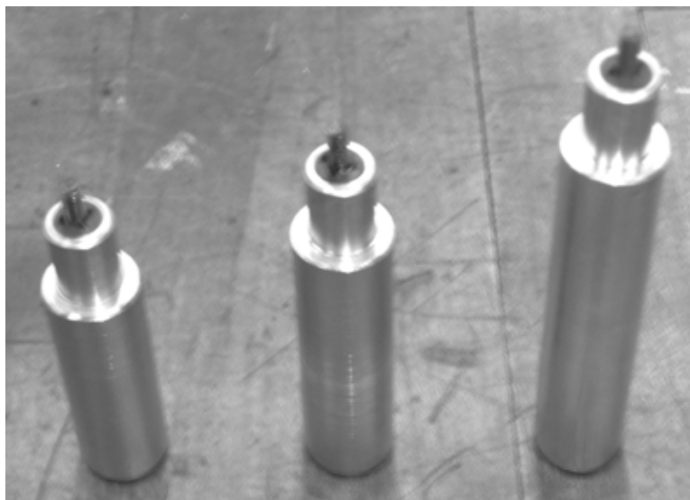
Figure 3-8. The three larger legs are used with the large cutting machine for the three larger casing diameters.
