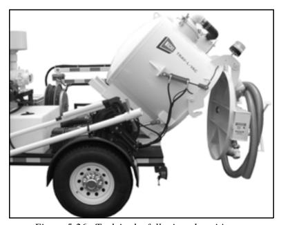
Figure 5-26. Tank in the fully tipped position.
