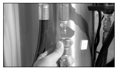
Figure 4-8. Connect the sprayer hose to the input fitting on the water heater.
