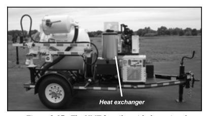
Figure 3-17. The VMT-2 trailer with the optional water heater.
