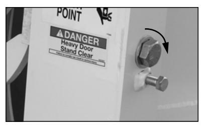
Figure 7-29. Turn the adjustment screw clockwise to tighten the latch.
