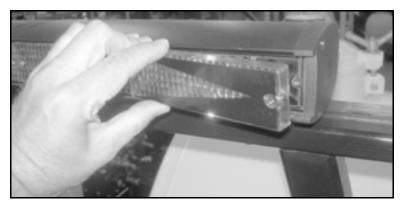
Figure 7-33. Remove the two screws and pull the cover off the burned-out bulb.
