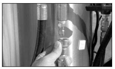
Figure 5-58. Connect the hose from the reel to the inlet on front of the water heater.
