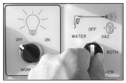
Figure 5-39. Turn the Vacuum/Pressure Washer switch OFF when finished spraying.
