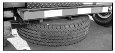
Figure 3-16. The spare tire is mounted beneath the back of the trailer on a cable mechanism. To remove the tire, turn the cable drive nut with a 3/4" wrench or socket until the tire is on the ground.
