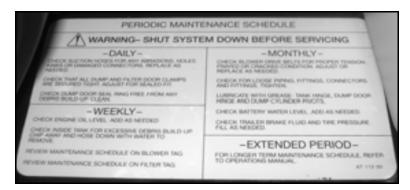
Figure 2-12. This label is on the trailer deck next to the engine. Shut the system down before performing service. (Part no. 67-112-00.)
