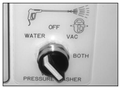
Figure 4-2. Turn the pressure washer switch to the WATER position.
