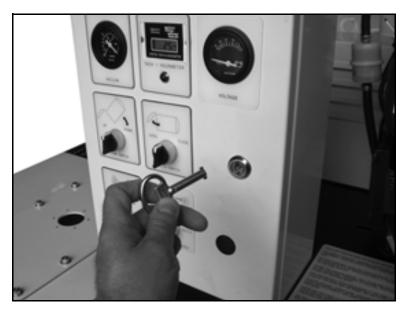
Figure 7-7. Insert the key and turn to open the control panel cover.
