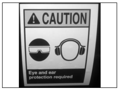
Figure 2-1. The eye and ear protection label is on the vacuum filter cover, right-hand side of the blower belt guard, and on the door of the spoils tank (3 locations). Wear protective gear when operating the vacuum system. (Part no. 77-160-05.)
