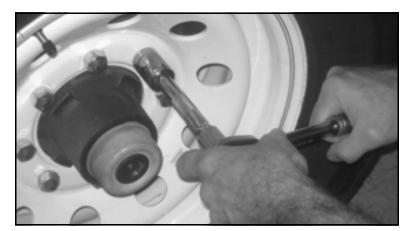
Figure 7-3. Remove the lug nuts.
