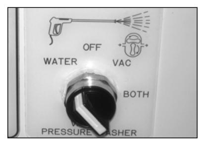
Figure 5-51. Turn the pressure washer switch to the WATER position.
