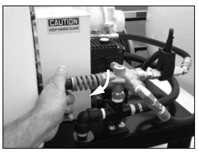
Figure 5-44. Turn the unloader knob clockwise to increase the water flow.
