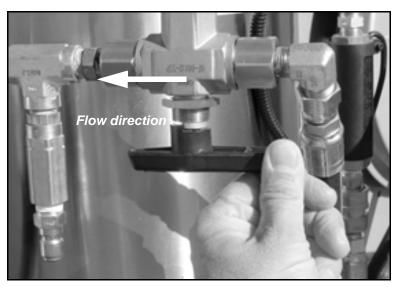
Figure 5-56. Set the water flow direction to the left to heat the tank water. (This setting disables the sprayer.)
