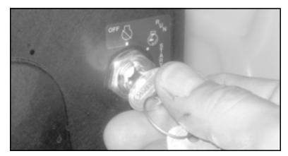
Figure 5-5. Turn the engine key to START. Release it to RUN when the engine starts.
