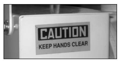
Figure 2-4. This caution label is on the left-hand side of the pressure washer belt guard. Keep hands away from the belt drive area while any equipment is operating or the gas engine is running. (Part no. 77-160-11.)
