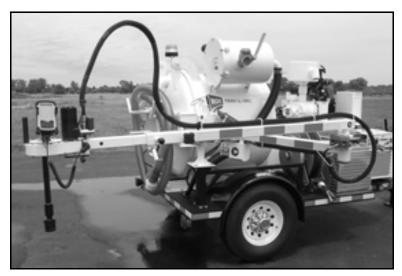
Figure 3-18. The ERV-750 valve exerciser extends on a pivoting, telescoping arm.
