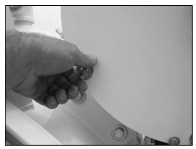
Figure 6-2. Loosen the wing nuts securing the filter canister cover.
