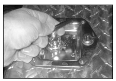
Figure 5-3. Lift the handle and turn it to open the job box.
