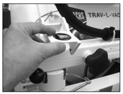
Figure 5-62. Lift the latch up and over the arm.
