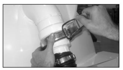
Figure 5-10. Insert the hose fitting into the inlet port and attach it with the locking collar.
