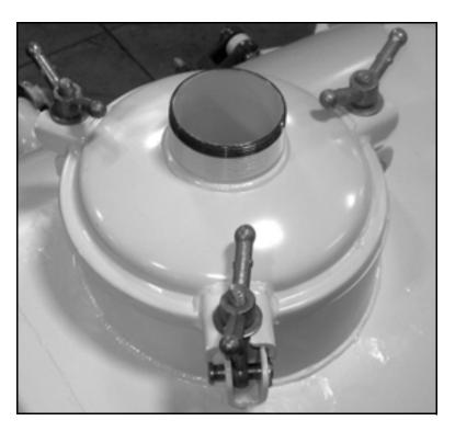
Figure 7-4. Loosen the wing nuts on the tank cap, then pull the cap off. It may be necessary to tap the side of the cap with a rubber hammer to break the seal.
