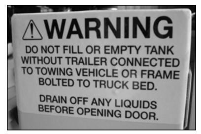
Figure 2-2. This warning label is on the right-hand side of the blower belt guard. Keep the trailer connected to the vehicle when operating the vacuum system. Drain liquids through the drain valve before opening the door to dump the tank. (Part no. 67-113-00.)
