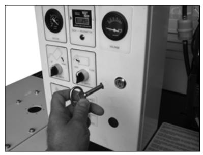
Figure 7-14. Insert the key and turn to open the control panel cover.
