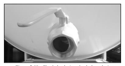
Figure 5-19. Check the drain valve before closing.
