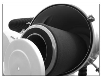
Figure 6-5. Remove the filter and take off the cover.
