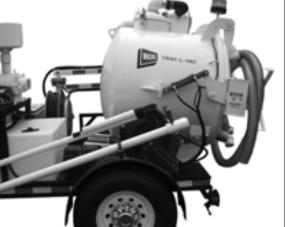
Figure 5-17. Turn the Dump Switch to the UP position and hold it **just until the tank has cleared the deck and begins to tip.** Tip the tank approximately 10° - 20°.
