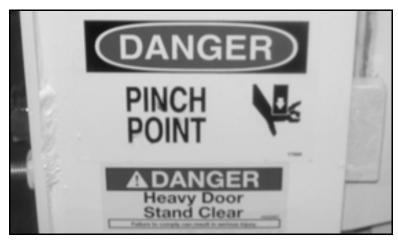
Figure 2-5. These danger labels are on both sides of the spoils tank at the door latches. Keep clear of the door when opening or closing it, or moving the tank. (Part no. 77-160-10 [above] and 77-160-25 [below].)
