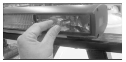
Figure 7-34. Remove the light bulb from the socket.
