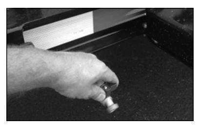
Figure 4-12. Open the drain valve on the back of the trailer to drain the water tank.
