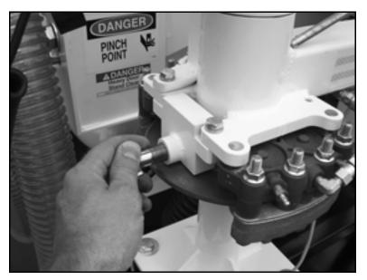
Figure 5-63. Loosen the set bolt to move the arm.
