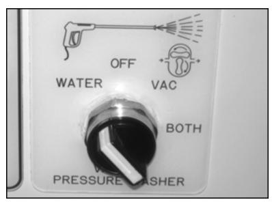
Figure 5-43. Turn the pressure washer switch to the WATER position.
