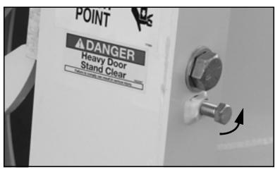
Figure 7-28. Turn the set screw counter-clockwise to loosen it.
