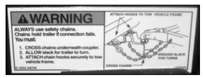
Figure 2-11. The safety chain warning label is on the tongue of the trailer. (Part no. 77-160-20.)
