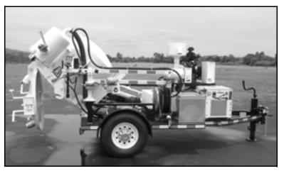
Figure 3-7. The tank dumping mechanism moves the tank to the rear of the trailer, opens the door latch, and tips the tank for dumping.
