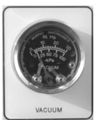
Monitor the pressure on the vacuum gauge while operating the vacuum.
