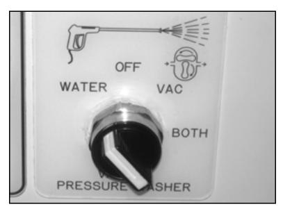
Figure 4-11. Turn the pressure washer switch to the WATER position.
