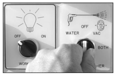
Figure 5-30. Turn the Vacuum/Pressure Washer switch OFF to turn off the vacuum.
