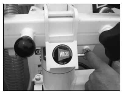
Figure 5-61. Pull the pin to release the latch.
