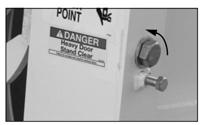
Figure 7-30. Turn the adjustment screw counter-clockwise to loosen the latch.
