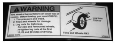
Figure 2-9. This warning label is on the trailer fender. Prior to each use of the trailer, check tire condition and lug nut tightness. (Part no. 77-160-15.)
