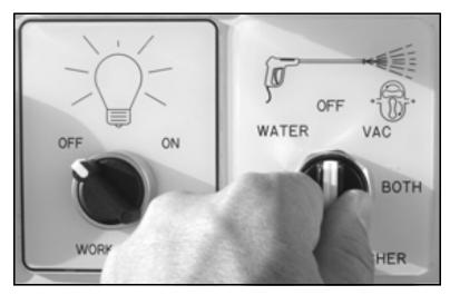
Figure 6-1. Turn the Vacuum/Pressure Washer switch to the OFF position.
