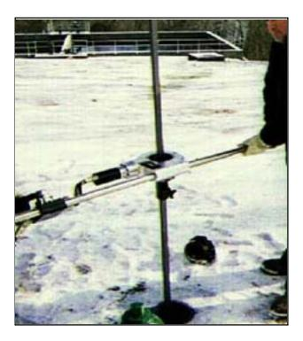
An extension handle is provided with each RS-2. It is designed to be inserted into the end of the handle assembly near the powerhead. A convenient quick release pin attached to the extension handle is inserted through the handle and extension to secure them.
