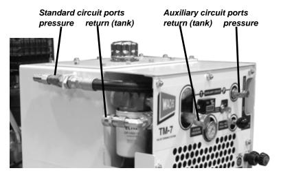
Figure 3-1. Connect the hydraulic hoses to **only one** circuit on the HPU.
