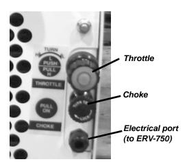
Figure 1-3. The photo shows the front panel engine controls.
