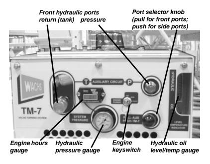
Figure 1-2. The photo shows the HPU front panel.
