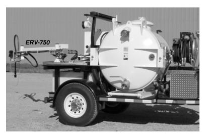
Figure 1-1. The photo shows the ERV-750 mounted on the Wachs Swivel Vac trailer.
