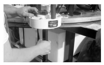
Figure 3-4. Insert the valve key adapter up through the bottom of the head.
