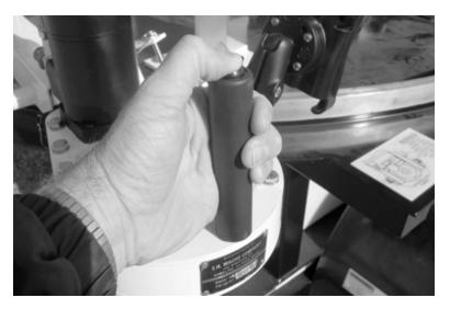
Figure 3-2. Hold down the brake release button to move the ERV-750 arm.
