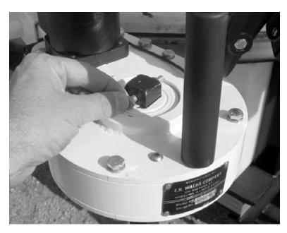
Figure 3-5. Put the bolt through the top of the valve key adapter and screw on the nut to secure it.
