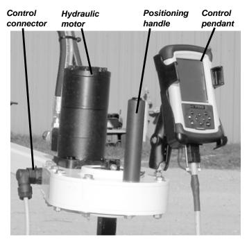
Figure 1-3. The photo illustrates the ERV-750 head.
