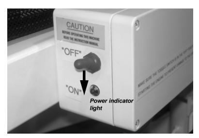
Figure 3-7. Push the switch on the control box to the "ON" position.
