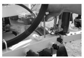
Figure 3-1. Release the two latches that secure the ERV-750 arm to the trailer.
