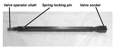
Figure 1-4. The telescoping valve key can be extended by pressing in the locking pin and pulling out the valve socket shaft.
