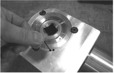
Figure 4-12. Tighten the 2 set screws to secure the sensors in place.
