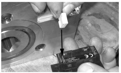
*Figure 4-4. Plug the connector into the pin block on the back of the counter.*
