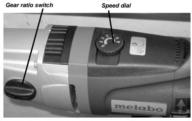
Use the speed control dial and the gear ratio switch to set the electric drive speed.
