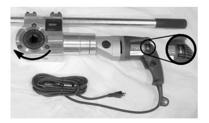
*Figure 1-3.* The photo illustrates the direction of rotation for indicated motor direction.
