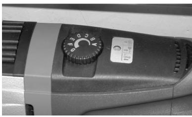
*Figure 3-4. Start with the speed dial set to the lowest speed ("A").*
