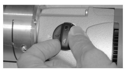
*Figure 3-6. Turn the gear ratio switch to the speed range desired.*
