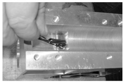
Figure 4-7. Remove the sensors.
