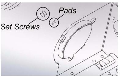
*Figure 4-8. Verify pad placement, there is no need to remove the clamping pads.*
