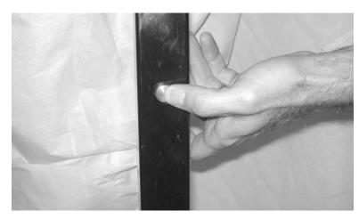
Figure 3-1. Press in the locking pin to adjust the length of the valve key.
