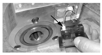
*Figure 4-3. Pull the connector from the back of the counter.*
