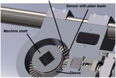
Figure 4-11. Cross section of assembly showing sensors against magnet retaining sleeve.
