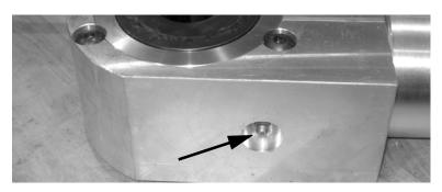
*Figure 4-1. Apply grease through the grease fitting on the head.*
