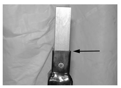
Figure 3-3. The valve operator rests on the shoulder at the top of the key shaft.
