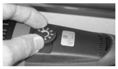
Figure 3-5. Turn the speed dial to increase the speed.
