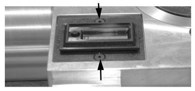
Figure 4-2. Remove the 2 screws to take the counter out of the head.
