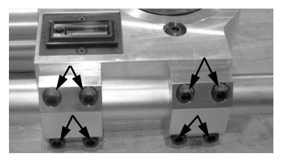
*Figure 4-5. Remove the 8 screws holding the handle to the head assembly.*
