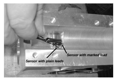
Figure 4-10. Insert the two sensors into the holes leading into the machine shaft cavity.
