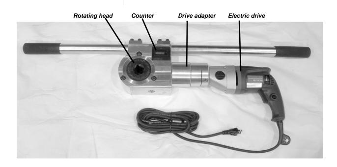
Figure 1-1. The photo illustrates the major components of the valve operator.
