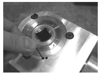
*Figure 4-6. Loosen the 2 screws holding in the sensors.*
