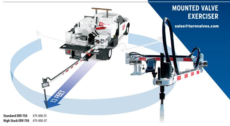
ERV-750 Automated Extended Reach Valve Operator, features Wachs hands free operation with Intelligent Automation. The extendable arm provides the full 750 ft/lbs of torque, even when fully extended. The support system utilizes dual pivot points to reach over to any curbside valve box or hydrant. Locking disc brake holds the full torque of the machine while operating. Frame is heavy duty 3in square steel tube construction. System includes a mechanical lock securing the machine during travel.
