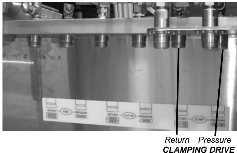
Figure 5-5. Connect the clamping drive hoses to the TCU (for machines with hydraulic clamping mechanism).
