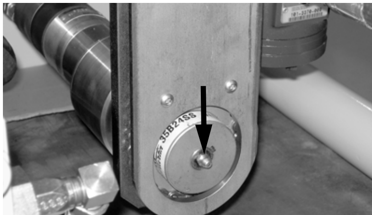
Figure 6-6. Grease the feed gearbox fitting.
