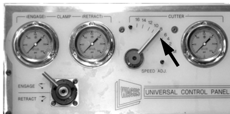
Figure 5-13. Push the cutting speed lever up slowly until the saw motion begins.
