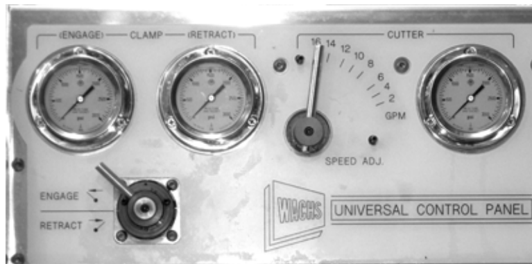
Figure 5-15. Set the cutting speed lever to the desired cutting speed.
