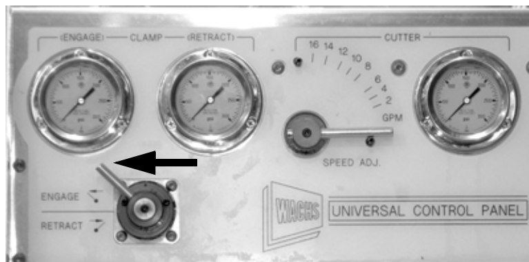
Figure 5-23. When the clamp has been retracted, move the clamping direction lever back to the ENGAGE position.
