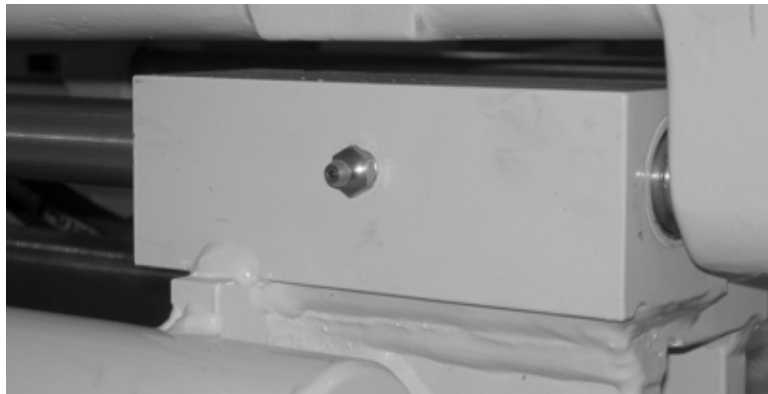
Figure 6-1. The guide shaft blocks on both sides of the saw frame have grease fittings.
