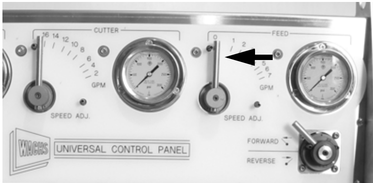
Figure 5-17. Stop the feed motion by setting the feed speed lever back to 0.
