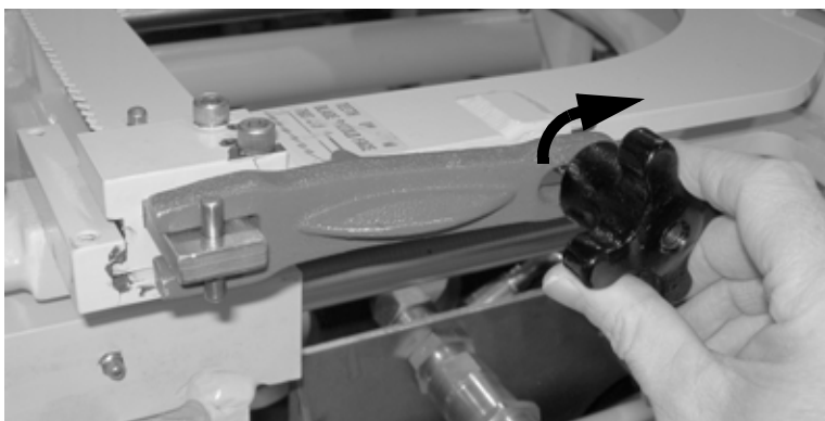
Figure 6-19. Turn the blade tensioning knob clockwise to tighten the blade.
