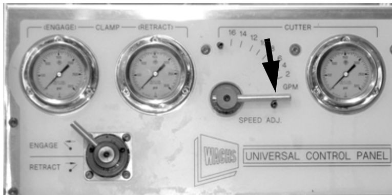
Figure 5-11. Set the cutting drive speed lever to 0 before starting the saw.
