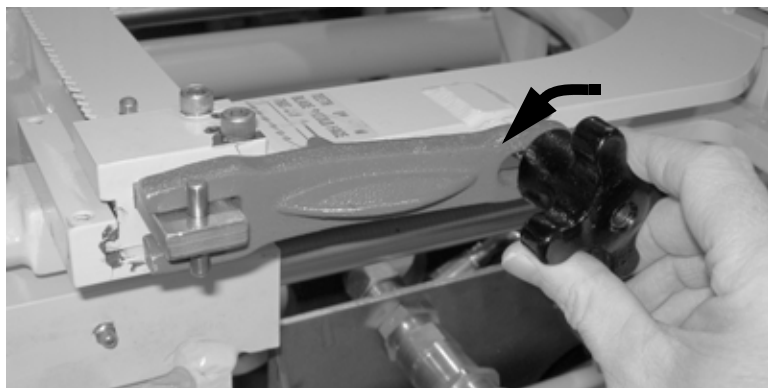
Figure 6-15. Turn the blade tensioning knob counter-clockwise to loosen the blade.
