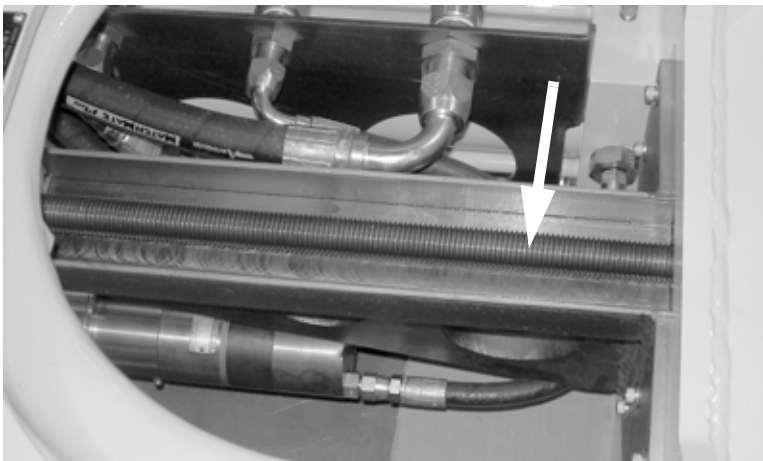
Figure 6-13. Grease the feed screw.
