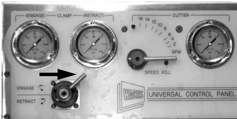
Figure 5-20. Set the clamping direction lever to the RETRACT position.
