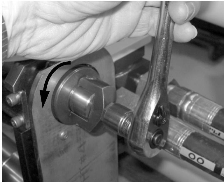
Figure 6-14. To retract the bow manually, flip the feed nut clevis out and turn the nut counter-clockwise using a 5/8" wrench or socket.
