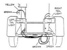
Figure 3-3. Wire the tail lights as illustrated.
