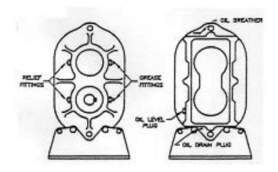
Figure 4-1. The diagram illustrates the blower components.
