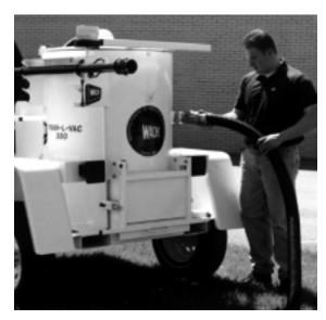
Figure 3-4. Connect the suction hose to the vacuum inlet port.
