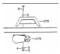
Figure 3-2. Assemble the fenders, frame, and axle as shown.
