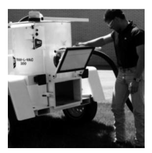
Figure 3-7. Open the dump gate to remove solid debris from the tank.
