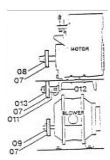
Figure 4-4. Adjust the belt tension by rotating the tensioning shaft (ref. 012).
