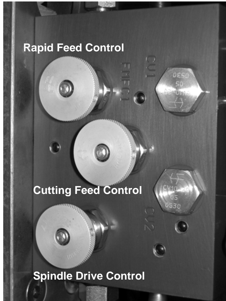
Figure 5-18. Use the knobs to adjust the flow control valves for the drives.
