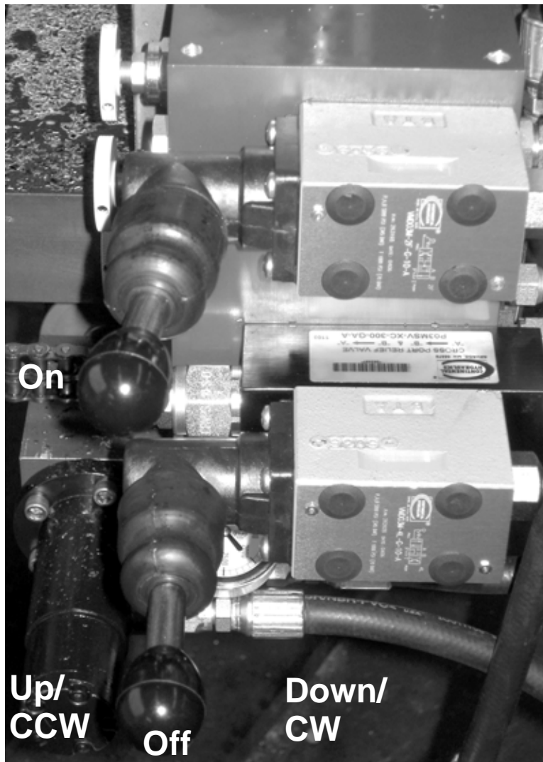
Figure 5-17. The spindle (cutting) drive is on the top in this orientation (on the shorter manifold block). The motion drive lever is on the bottom (on the taller manifold block).
