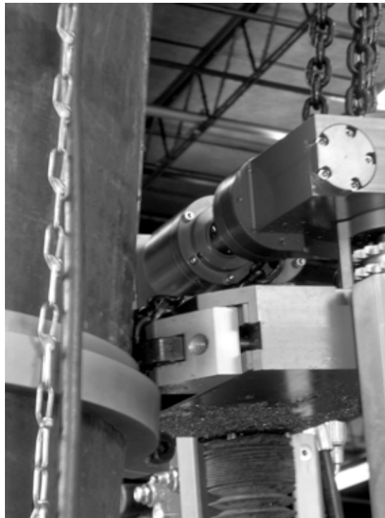
Figure 5-8. Set the top of the machine against the pipe, with the tracking wheels on against the pipe and on top of the guide ring.
