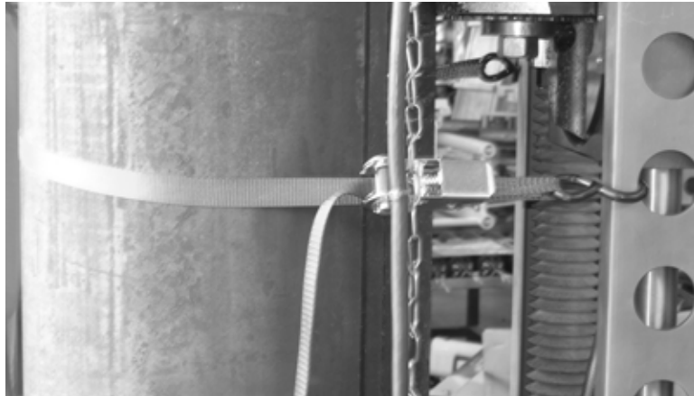
Figure 5-9. Use a binding strap around the pipe and center of the machine to pull it snug against the pipe.
