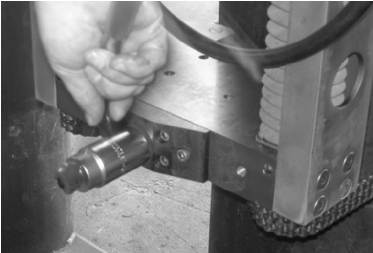
Figure 5-12. Turn the bottom tensioning nut counter-clockwise to tighten the chain.
