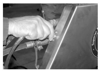
Figure 3-10. Attach a water hose to the coolant fitting.
