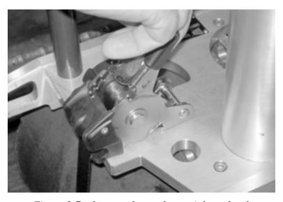
Figure 3-7. Operate the ratchet to tighten the clamping strap.
