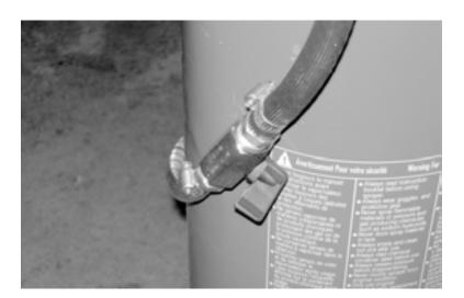
Figure 3-15. The coolant spray tank has an on-off valve on the hose.
