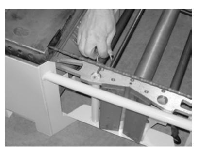
Figure 3-26. Put in the locking pin to secure the machine in the storage frame.
