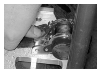
Figure 3-24. Press the button on the clamping ratchet to release the strap.
