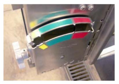
Figure 4-1. Fully release the tension on the wire.
