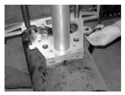
Figure 3-6. Wrap the clamping strap around the pipe and fasten the hook through the hole as shown.
