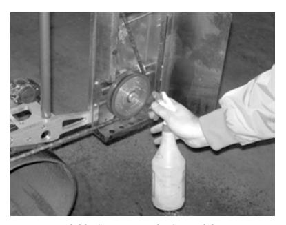
Figure 3-23. Spray water-displacing lubricant on moving parts before storage.
