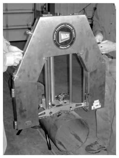
Figure 3-3. Set the machine on the pipe, with the wire on the fall-off side of the cut.
