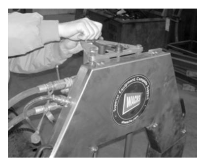
Figure 3-16. Turn the feed handle to advance the wire into the pipe.
