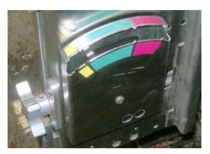
Figure 3-17. Operate the feed handle to keep the tension gauge indicator in the green band.
