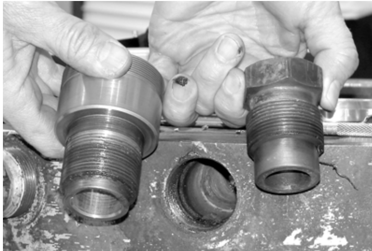
Figure 3-2. Select the gland adapter (left) to match the hole and thread size of the gland nut (right).
