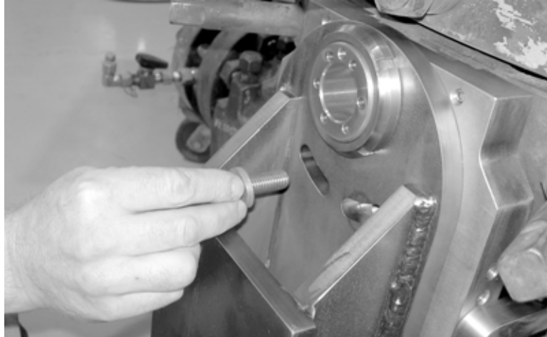
Figure 3-9. Insert the base mounting bolts into the threaded holes in the saddle.
