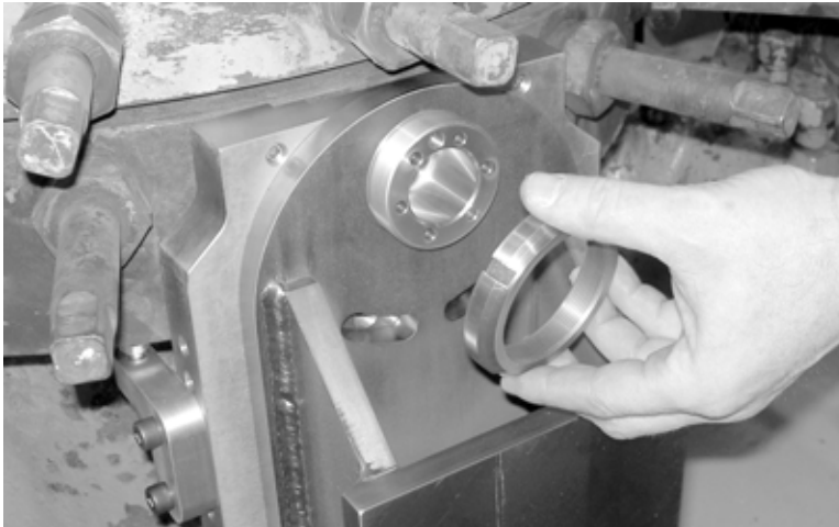
Figure 3-7. Fasten the base plate to the saddle by screwing the locking ring in place.
