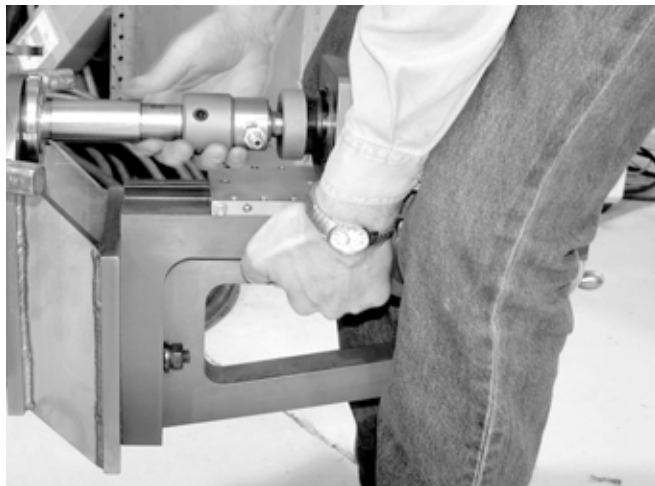
Figure 3-15. Lift the drill and slide so that the alignment shaft fits into the adapter. Feed the drill forward.
