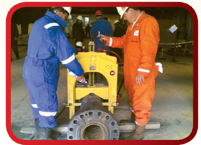
Guillotine saws feature fast, easy operation and the ability to cut most materials
