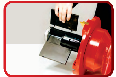
SDB 412 sets up quickly with self centering mandrel and quick change extension legs
