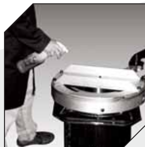
Re-install Split Frame on adapter ring and attach internal casing attachment.
