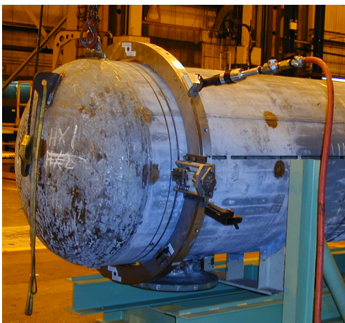
Figure 2 - Wachs LCSF split frame end cap removal
