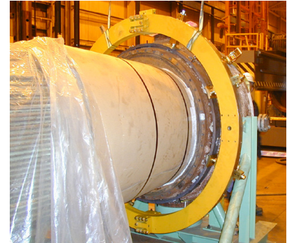
Figure 4 - Large diameter flange facing with HDSF split frame
