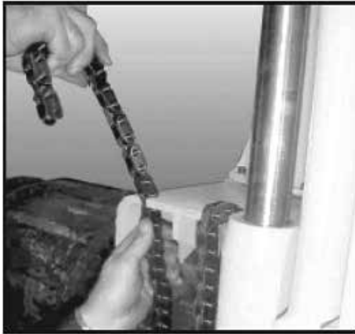
Figure 5-1. Fasten the clamping chain (or chains) around the pipe and through the clamping slot in the saddle.
