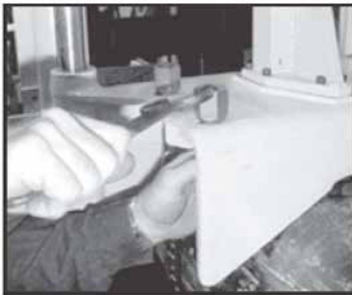
Figure 5-2. Tighten the chain clamping nut to secure the saw to the pipe.
