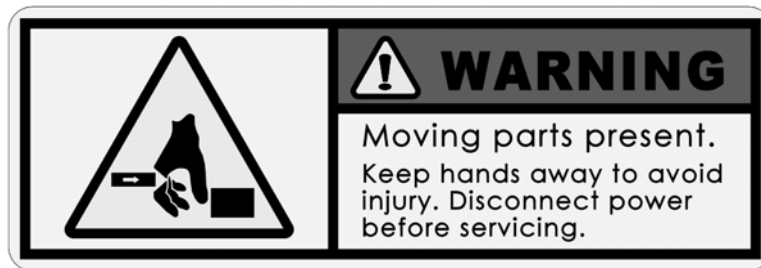
Figure 2-5. The moving parts warning label is attached in 2 places on the saw frame assembly. (Part no. 03-113-04.)
