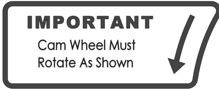
Figure 2-3. The cam wheel label is on the back of the main assembly, illustrating the direction of rotation. (Part no. 03-113-01.)
