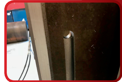
Heavy wall pipe can be cut by milling in multipole passes to preserve tooling life
