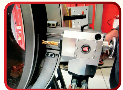
Milling head handwheel is used for plunge control and to set the cutting depth
