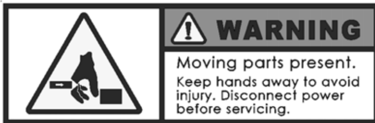
Figure 2-3. The Moving Parts warning label is on the trip assembly (part no. 03-113-04).
