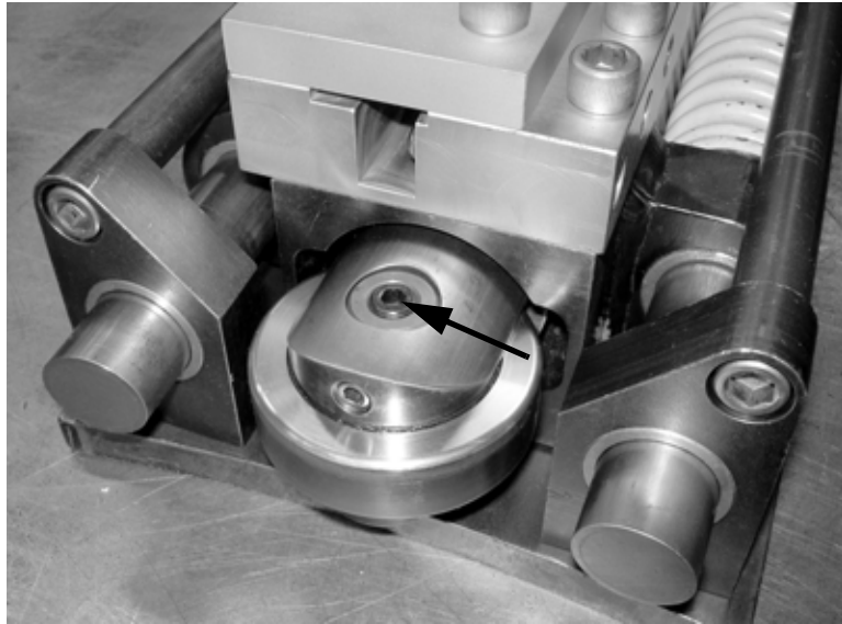
Figure 4-2. Remove the plug and install a grease fitting to grease the tracking wheel. After greasing the wheel, remove the grease fitting and replace the plug.
