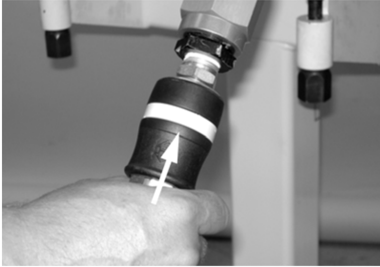
Figure 5-86. Push the air line disconnect onto the air drive fitting until it locks in place.
