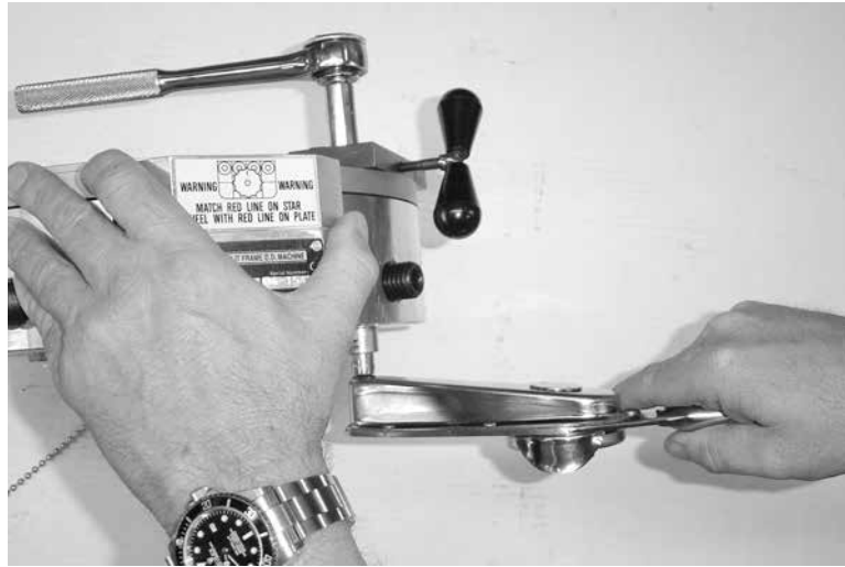
Figure 7-18. Secure the eccentric shaft.
