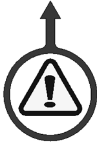
Figure 2-22. The alignment pin location label is attached to indicate the alignment pin holes. Two labels are on the LCSF, one for each pin location. (Part no. 60-1275-00.)
