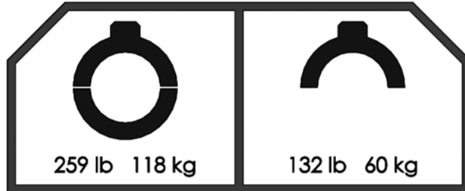
Figure 2-19. Weight labels for the LCSF are attached to the pinion housing. Weights and part no. vary according to LCSF model. (Part no. 60-1279-XX.)
