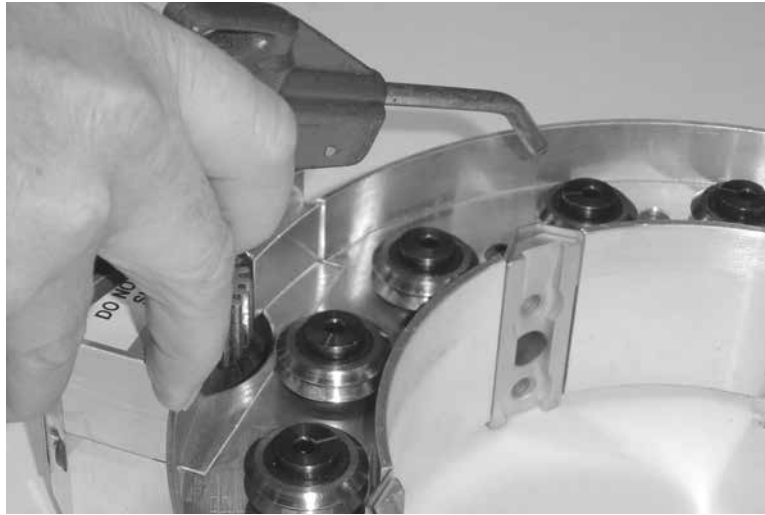
Figure 7-10. Clean debris from the stationary ring.
