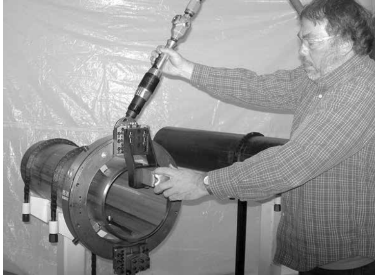
Figure 2-10. When using accessories that require you to operate their controls (shown with universal counterbore slide), stand in a position where you can operate the machine without contacting moving parts.
