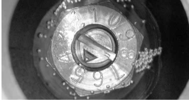
Figure 6-1. Use the needle valve screw to adjust the drip rate of the air motor oiler.
