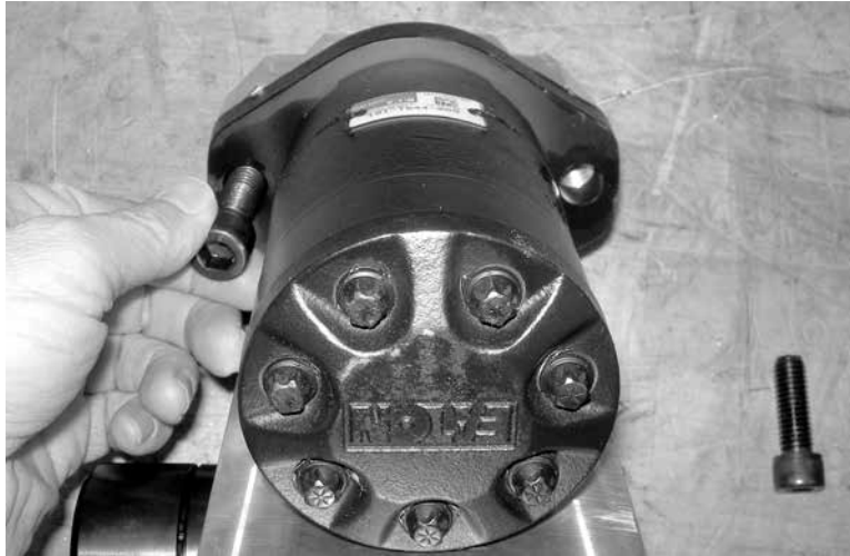
Figure 5-47. Remove the hydraulic drive screws to detach the drive motor from the adapter.
