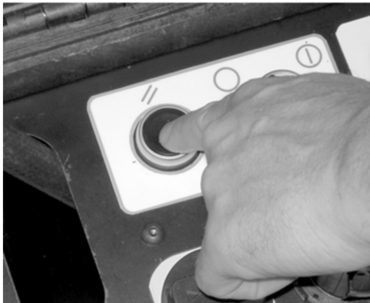
Figure 5-81. The Reset button resets the ACM after a loss of pressure or an emergency stop.
