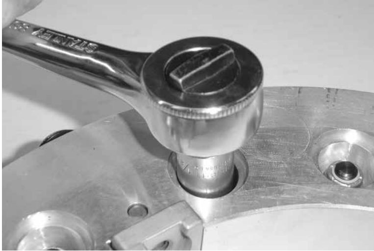
Figure 7-13. Loosen the lock nuts.
