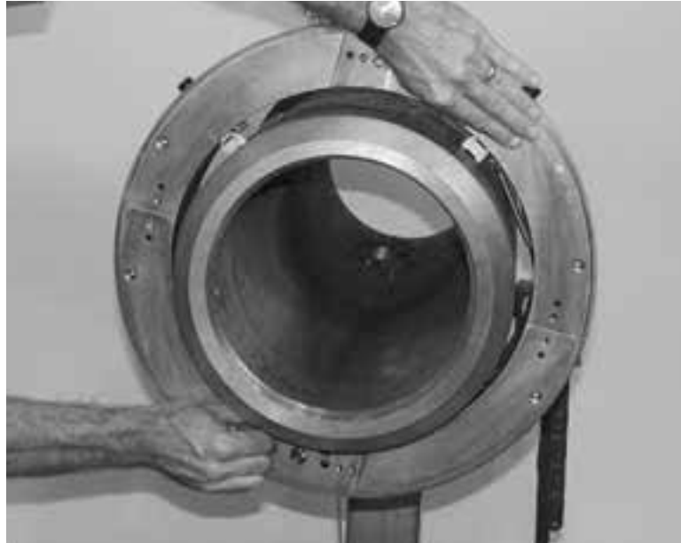
Figure 5-26. Rotate the machine by hand.
