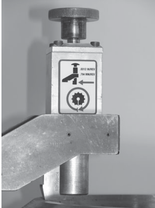
Figure 5-69. Axial (.0312) and radial (.0784) adjustment per revolution.
