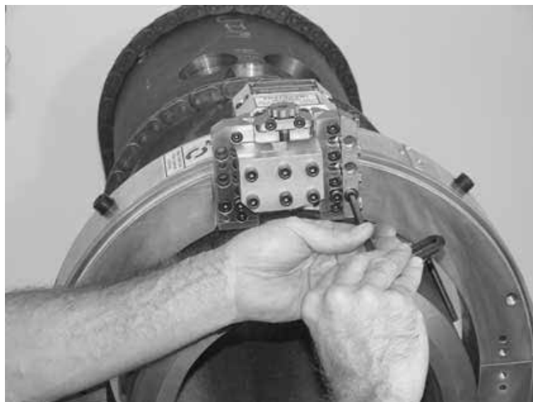
Figure 5-28. Tighten the SHCS on each side of the tool slide.
