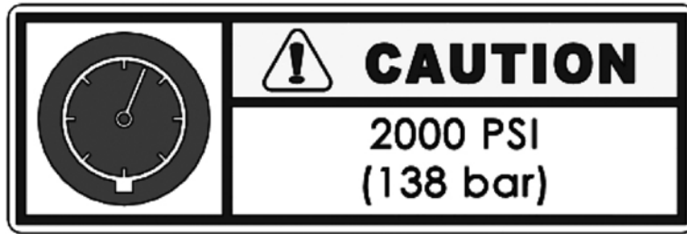
Figure 2-17. The hydraulic pressure label is attached to the LCSF hydraulic drive. Do not operate the equipment with greater than 2000 psi (138 bar) hydraulic pressure. (Part no. 90-402-01.)
