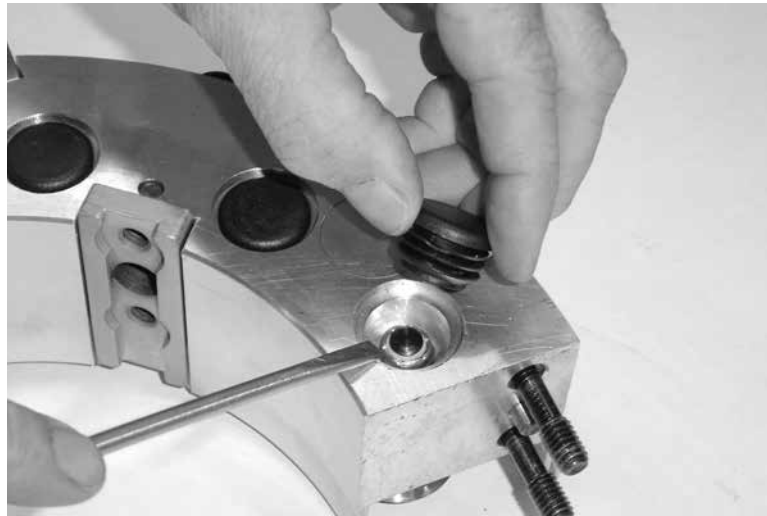
Figure 7-12. Remove the plastic caps to inspect the bearing assemblies.
