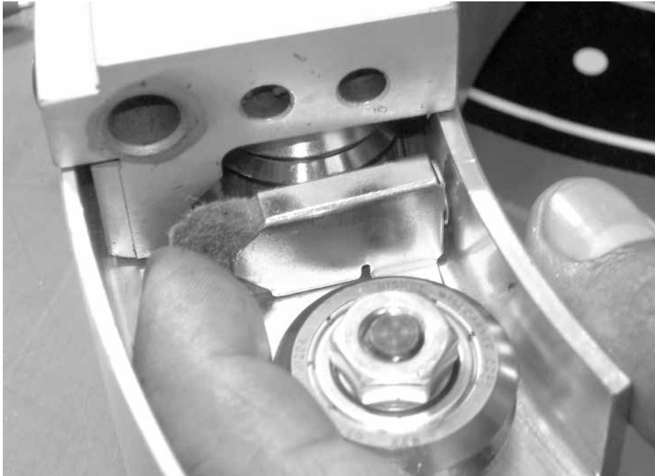
Figure 6-6. Push the wiper into the bracket and turn the rotating ring into position.
