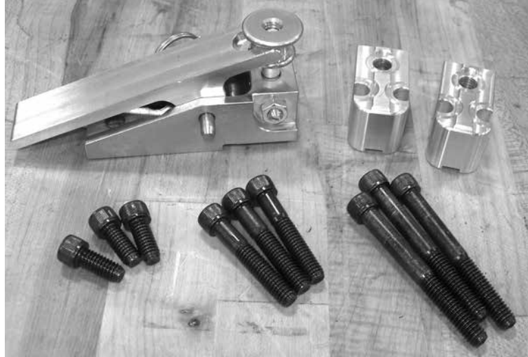
Figure 5-39. The trip assembly is provided with 2 extension blocks, and 3 sizes of screws for the 3 configurations (no block, 1 block, or 2 blocks).
