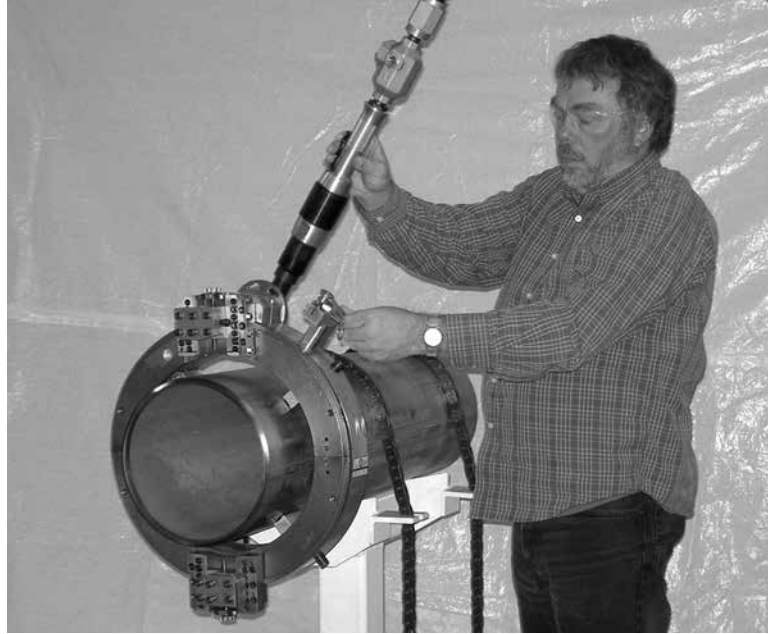
Figure 2-8. If possible, stand behind the LCSF to stay clear of moving parts while operating the controls.
