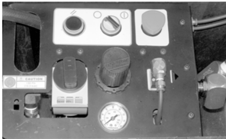
Figure 5-75. The ACM controls should be in the pre-operation state, as shown, before connecting the air lines.
