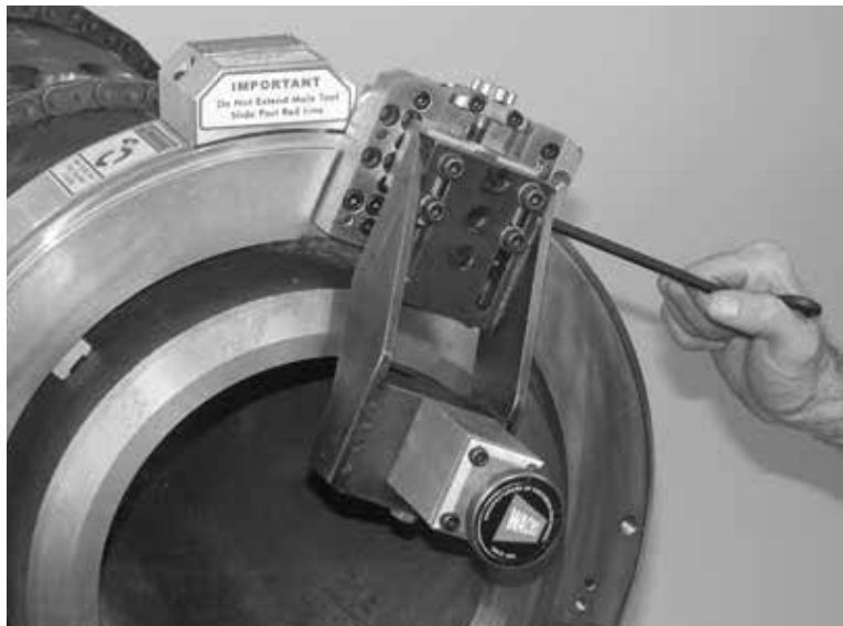
Figure 5-64. Secure the SCHS on the side of the bevel slide.
