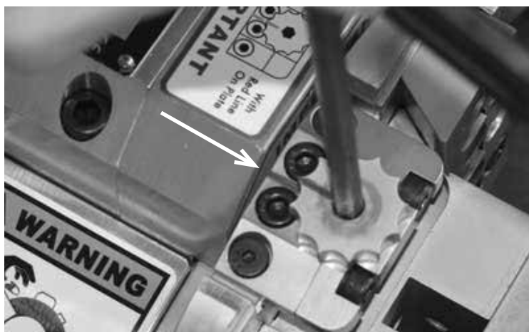
Figure 5-44. Time the starwheel. You can align any point of the wheel with the red line on the tool block.
