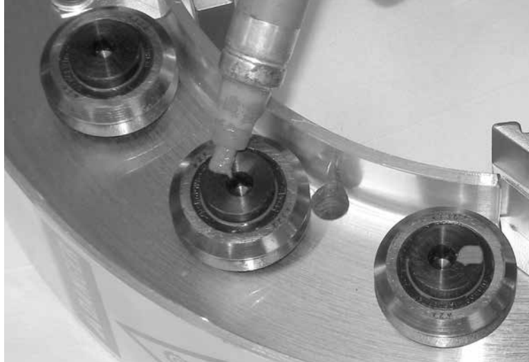
Figure 7-3. Mark the edge of each bearing.
