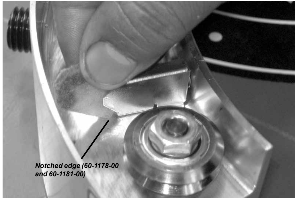
Figure 6-5. Replace the wiper in the bracket, with the notched edge down.
