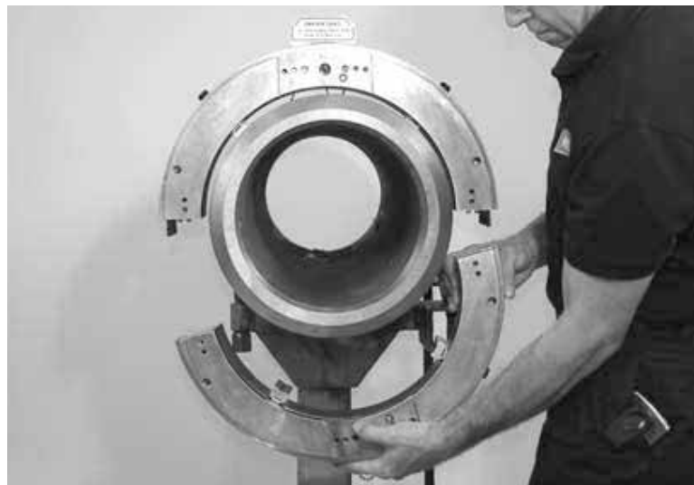
Figure 5-19. Fit the halves together on the pipe.
