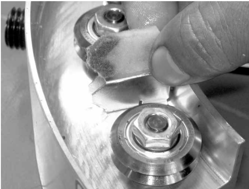
Figure 6-4. Inspect the wiper for wear, damage, or debris.
