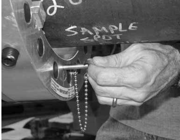
Figure 5-25. Remove the frame locking pins.
