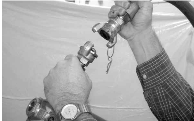
Figure 2-11. Disconnect pneumatic power by removing the air line from the pneumatic drive.
