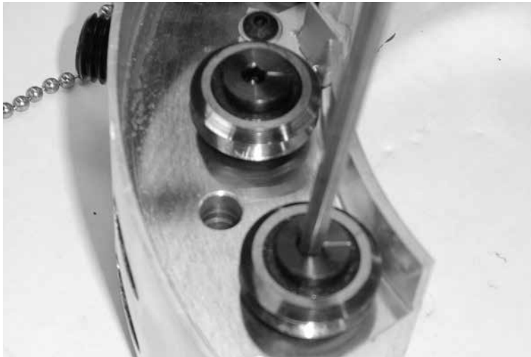
Figure 7-14. Set the marks on the eccentric shafts toward the center of the ring.
