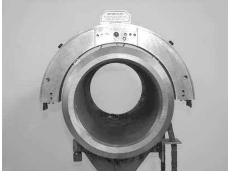
Figure 5-18. On horizontal pipe, set the side of the machine with the pinion housing on top of the pipe.
