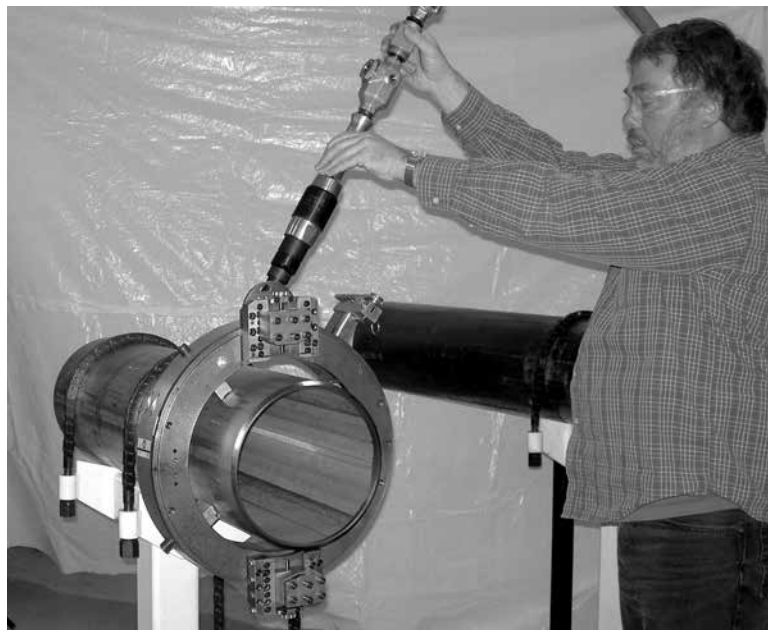
Figure 2-9. When operating the LCSF from the front, stand to the side of the machine to operate the controls without reaching across the rotating ring.
