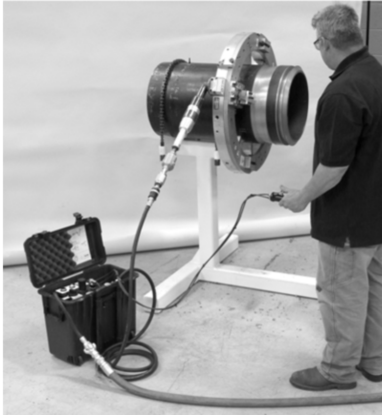
Figure 5-74. Position the ACM at a convenient distance from the split frame machine.
