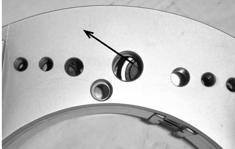
Figure 7-20. Check for bearing rotation as you turn the rotating ring.
