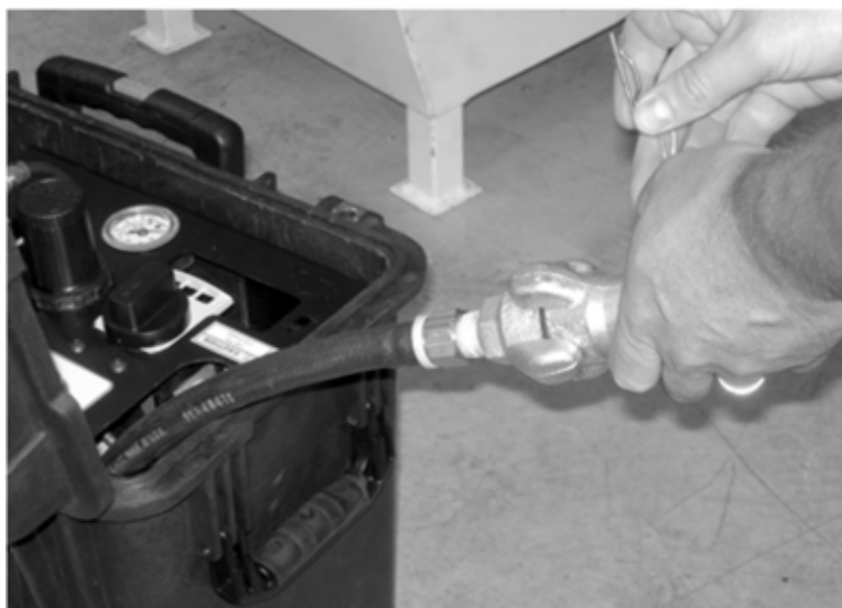
Figure 5-76. Connect the line from the air source to the input connector on the ACM.
