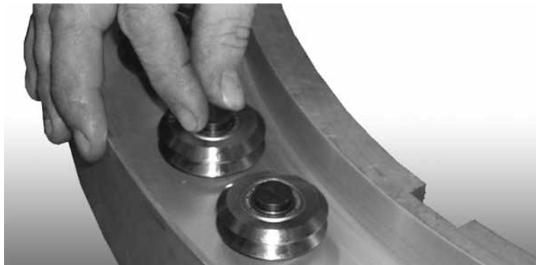
Figure 7-4. Rotate the eccentric shafts so that the high point of each bearing faces the inside of the ring.
