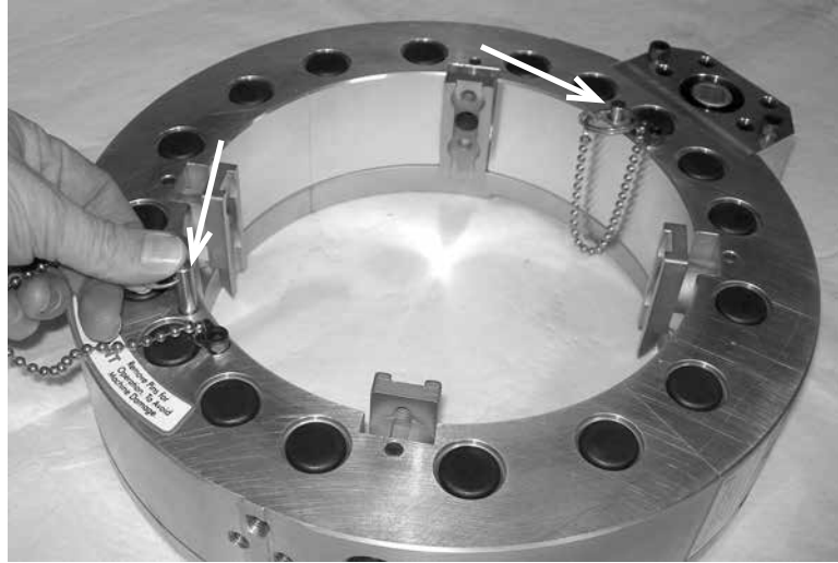
Figure 5-15. Insert the frame locking pins through the machine.
