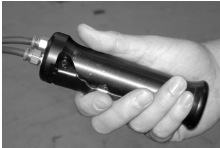
Figure 5-83. Squeeze the trigger on the handheld pendant to operate the machine.
