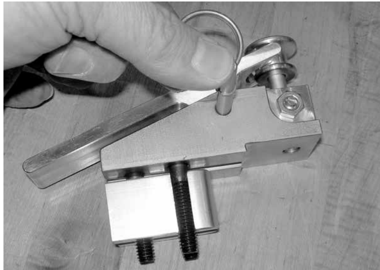
Figure 5-40. Pull out the pin and remove the trip lever.
