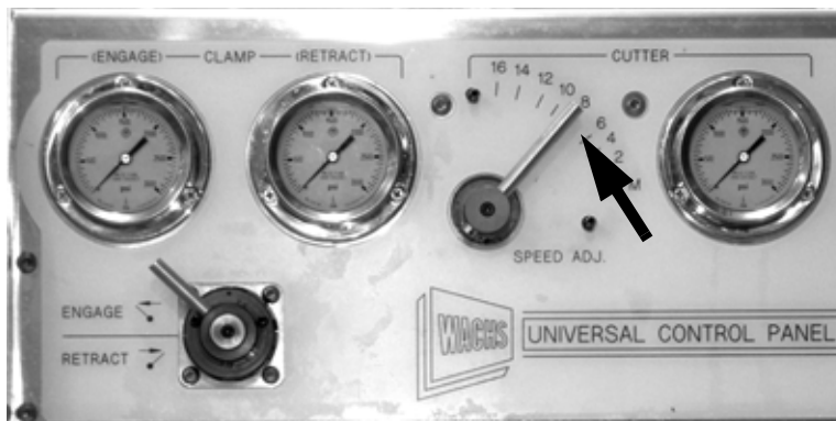
Figure 5-54. Push the cutting speed lever up slowly until the saw motion begins.
