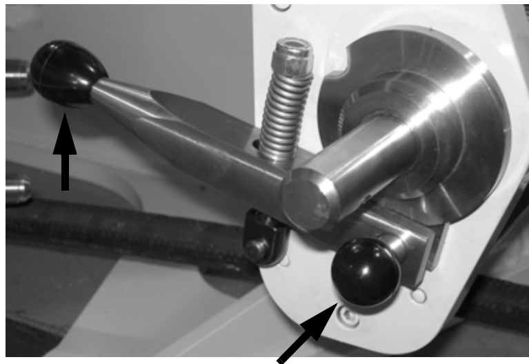
Figure 5-15. Push the feed lever up to the disengaged position and push in the lockout pin.
