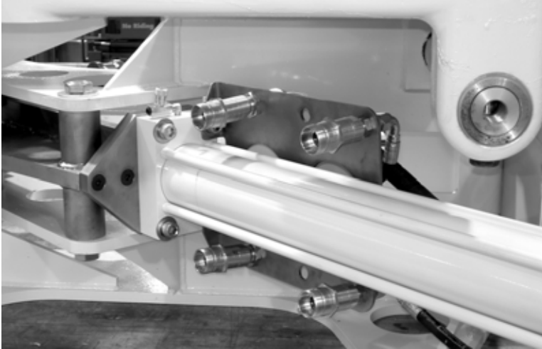
Figure 3-6. A hydraulic fitting bulkhead on the Goliath Guillotine has connectors for operating the autoclamp and cutting drives remotely from the TCU.
