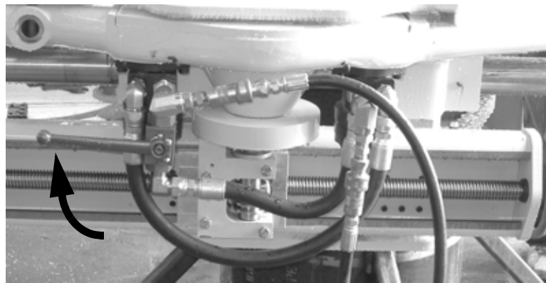
Figure 5-24. Open the flow valve (up position) to engage the saw cutting motion.
