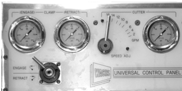
Figure 5-55. Set the cutting speed lever to the desired cutting speed.
