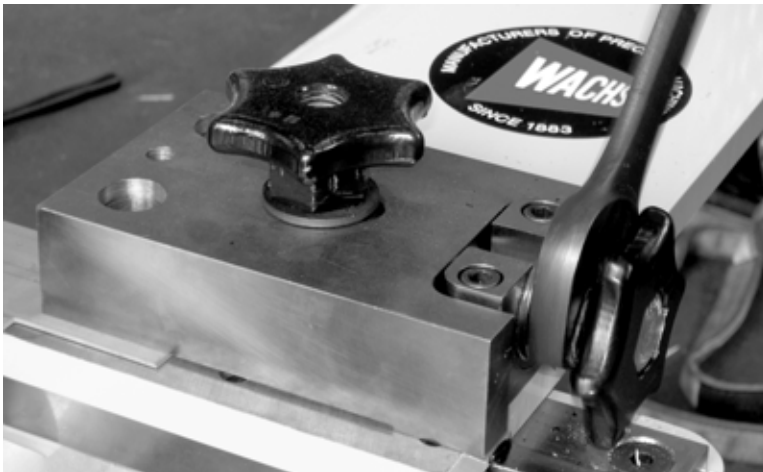
Figure 5-11. Tighten the tensioning knob to pull the saw blade tight.
