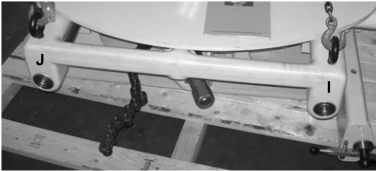
Figure 5-3. Eyebolts can be screwed into the threaded holes I and J in the end of the frame.
