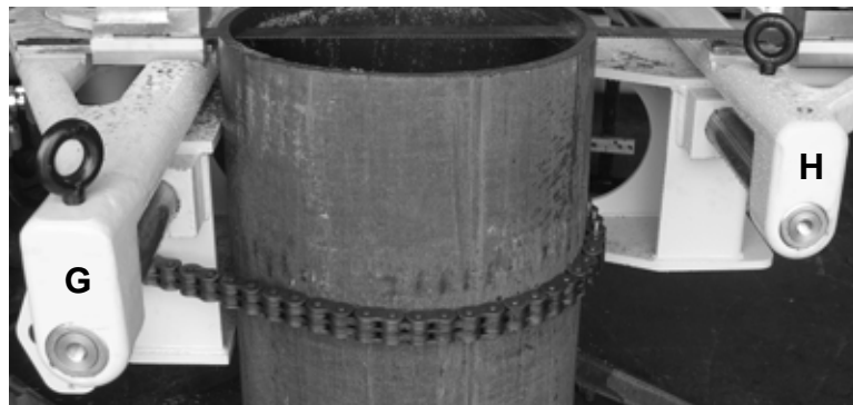
Figure 5-2. The eyebolts can be screwed into the threaded holes G and H on the end of the frame.
