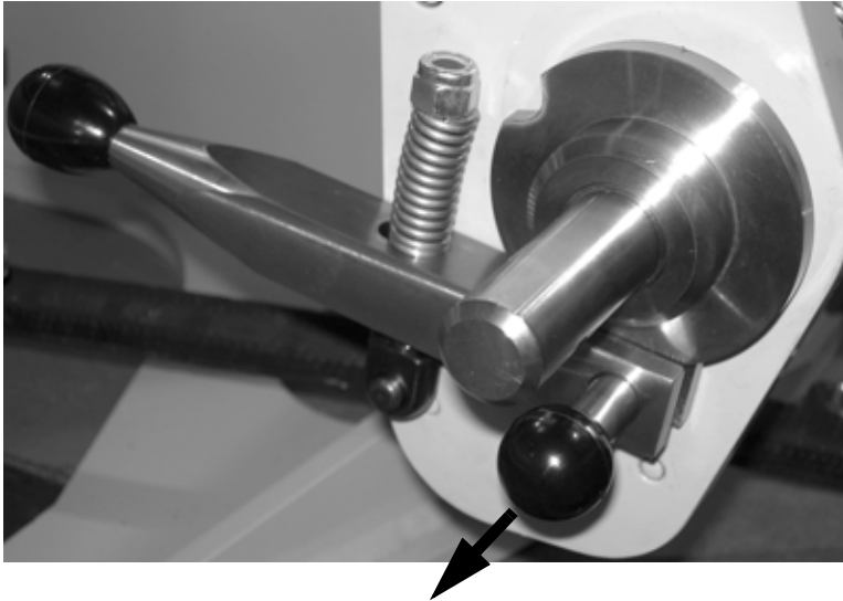
Figure 5-16. Pull out the lockout pin and release the feed lever to engage the autofeed.
