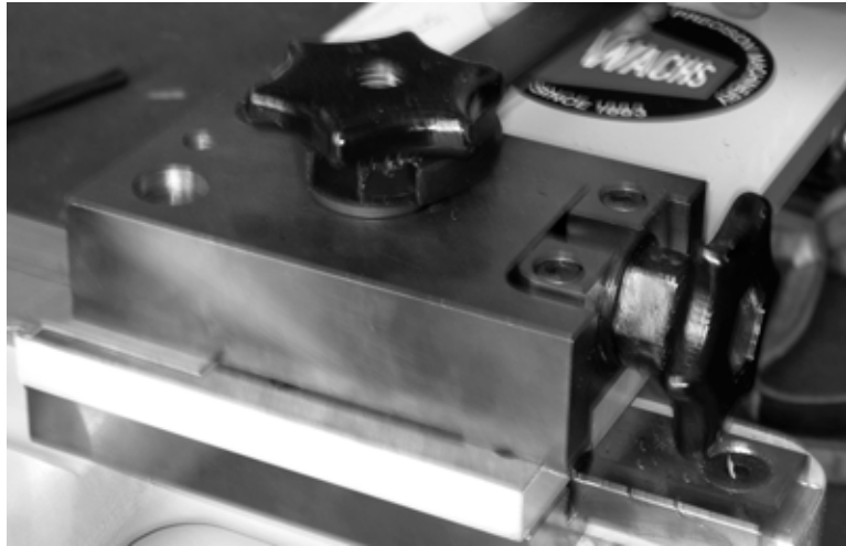
Figure 5-12. Tighten the clamp knob on both clamp blocks to secure the blade for cutting.
