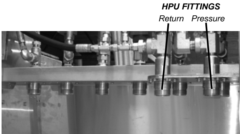
Figure 5-43. HPU hose fittings on the back of the control unit.
