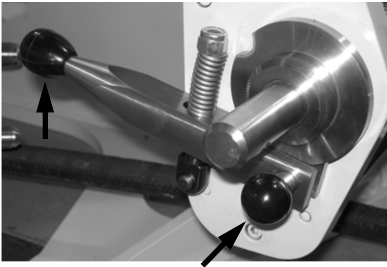
Figure 5-23. The feed lever should be disengaged and the lockout pin pushed in.
