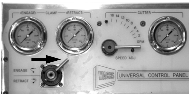
Figure 5-58. Set the clamping direction lever to the RETRACT position.
