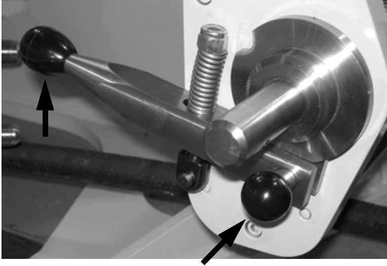
Figure 5-35. The feed lever should be disengaged and the lockout pin pushed in.
