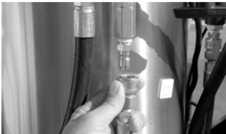
Figure 5-70. Connect the hose from the reel to the inlet on front of the water heater.
