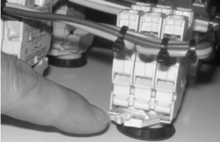
Figure 7-12. The locking ring shown holds the body of the switch to the front section.
