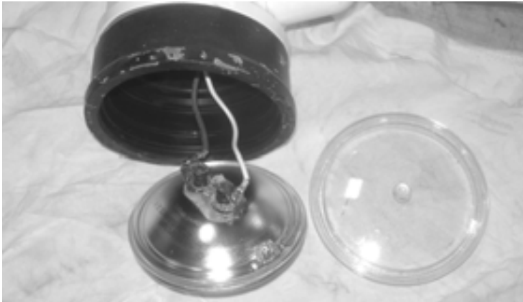
Figure 7-38. Pull the cover and bulb out of the rubber seal around the lamp housing.
