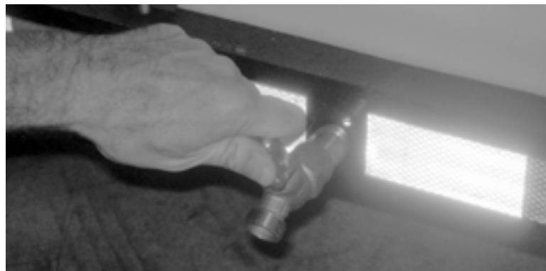
Figure 4-7. Open the drain valve on the back of the trailer to drain the water tank.
