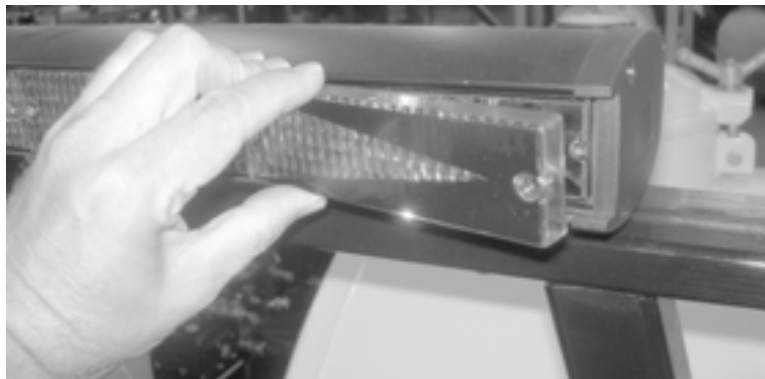
Figure 7-36. Remove the two screws and pull the cover off the burned-out bulb.
