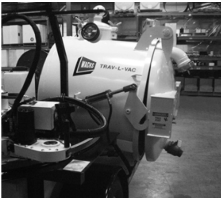
Figure 5-25. The tank door will swing open when the latches are released.
