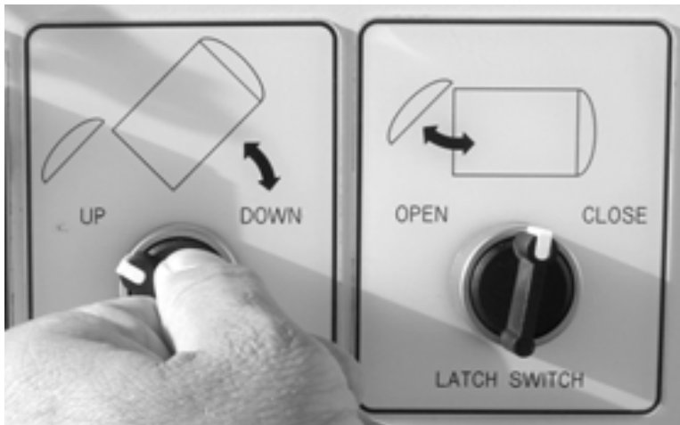
Figure 7-32. Turn the Dump Switch to the UP position and hold it until the tank is completely tipped.
