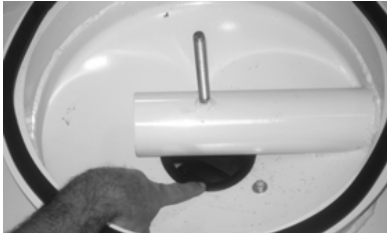
Figure 7-6. The seal is in the vacuum port. Pry the old seal out and press the new seal in.
