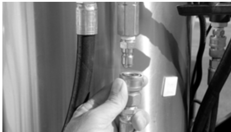
Figure 4-10. Connect the sprayer hose to the input fitting on the water heater.
