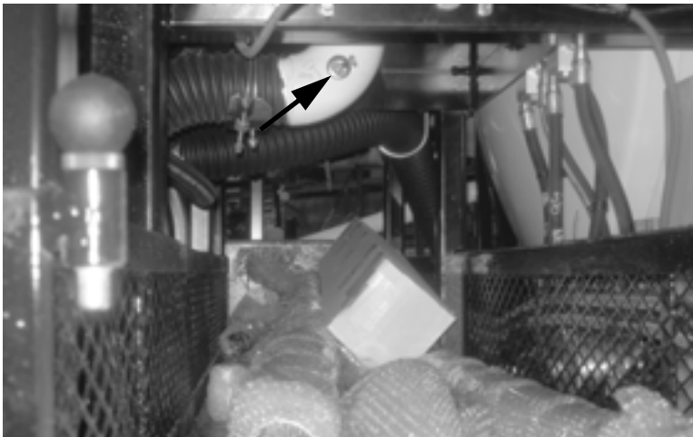
Figure 6-6. Access the blower lubrication port through the accessory storage box.
