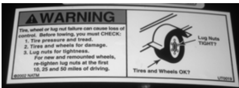
Figure 2-9. This warning label is on the trailer fender. Prior to each use of the trailer, check tire condition and lug nut tightness. (Part no. 77-160-15.)
