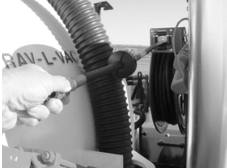
Figure 4-9. Pull a sufficient length of hose from the sprayer reel to reach the front of the water heater.
