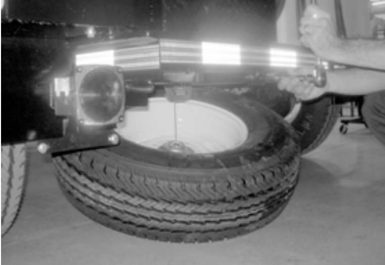
Figure 5-2. Turn the cable release nut to lower the spare tire to remove it.
