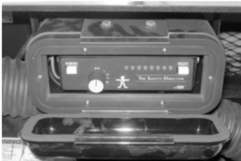
Figure 5-56. Pull the top of the enclosure cover forward to open it.
