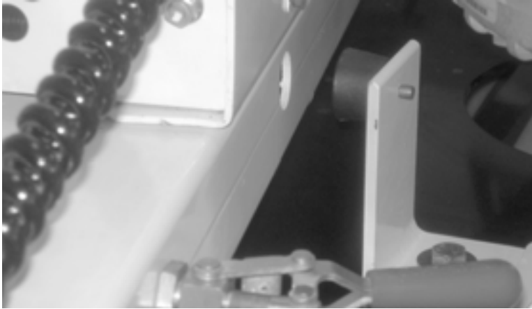
Figure 5-76. On trailers equipped with both a TM-7 and an ERV-750, a stop bracket with a rubber bumper prevents the TM-7 from swiveling too far.
