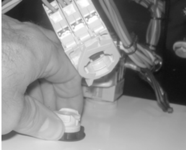
Figure 7-14. Remove the locking ring to take the front of the switch out of the control panel.
