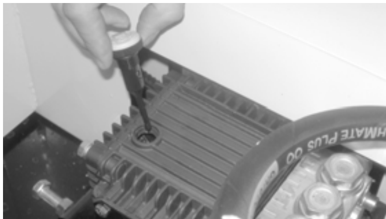
Figure 6-20. Remove the oil cap on the sprayer pump and fill the pump with oil. The cap has a dipstick.
