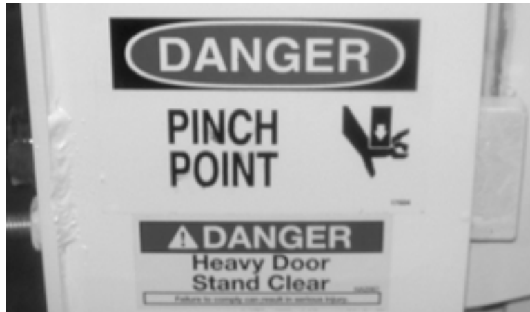
Figure 2-5. These danger labels are on both sides of the spoils tank at the door latches. Keep clear of the door when opening or closing it, or moving the tank. (Part no. 77-160-10 [above] and 77-160-25 [below].)
