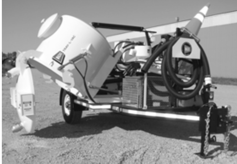
Figure 3-8. The tank dumping mechanism moves the tank to the side of the trailer, opens the door latch, and tips the tank for dumping.
