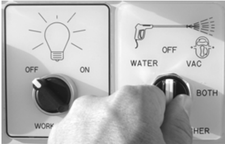
Figure 5-31. Turn the Vacuum/Pressure Washer switch OFF to turn off the vacuum.
