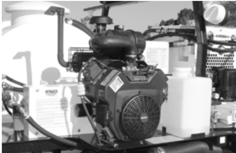
Figure 3-6. The gasoline engine, shown in the center, powers all of the equipment provided with the VMT-1.
