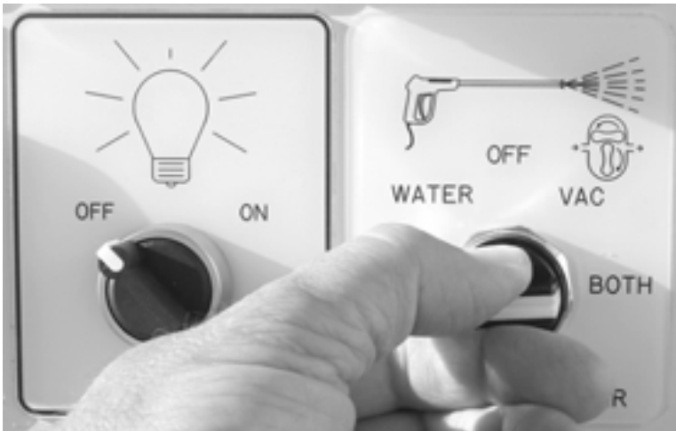
Figure 5-38. To use both the washer and vacuum, turn the Vacuum/Pressure Washer switch to the BOTH position.
