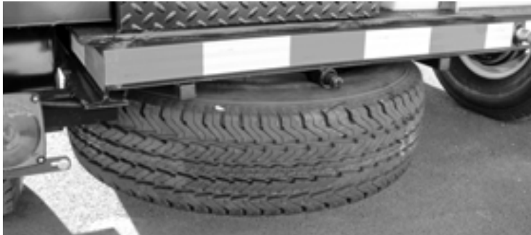
Figure 3-18. The spare tire is mounted beneath the back of the trailer on a cable mechanism. To remove the tire, turn the cable drive nut with a 3/4" wrench or socket until the tire is on the ground.
