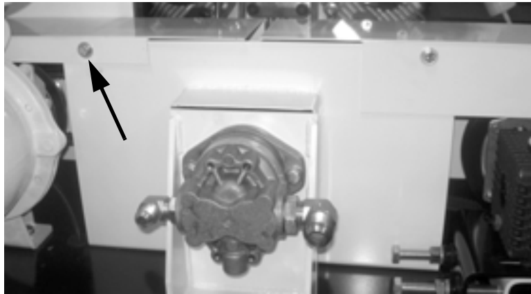
Figure 7-17. Remove the screw on the back of the blower belt cover.
