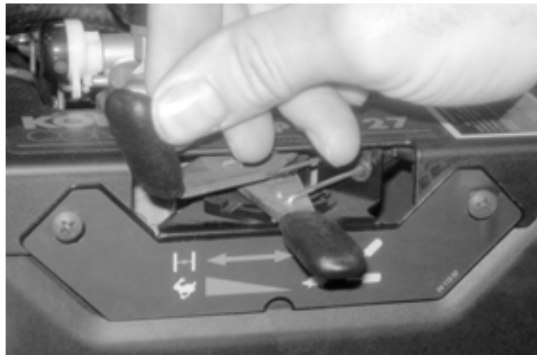
Figure 5-5. To start the engine, set the choke lever (top) all the way to the left, and the throttle lever (bottom) in the middle.
