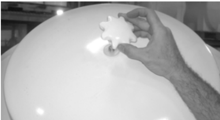
Figure 7-5. Remove the knurled knob from the tank cap, then pull the cap off. It may be necessary to tap the side of the cap with a rubber hammer to break the seal.
