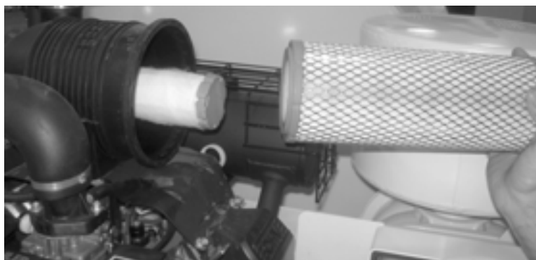
Figure 6-17. The filter has two elements. Check both and replace if dirty or clogged.
