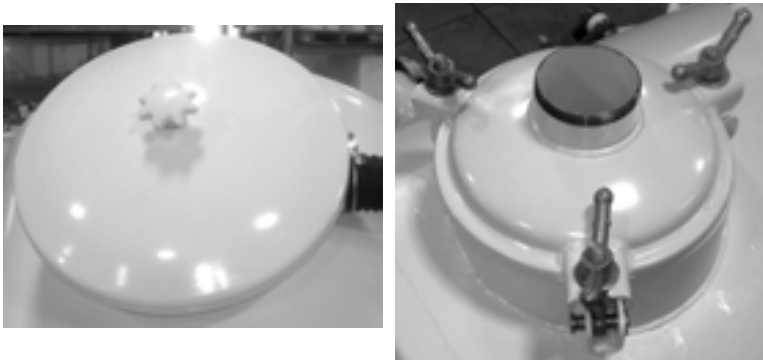
Figure 7-4. The older style of tank cap (left) has a knurled knob; the newer style (right) uses wing nuts.
