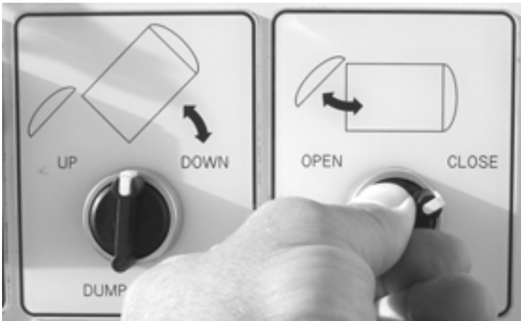
Figure 5-29. When the tank is in the down position, turn the Latch Switch to the CLOSE position until the latches are fully engaged.
