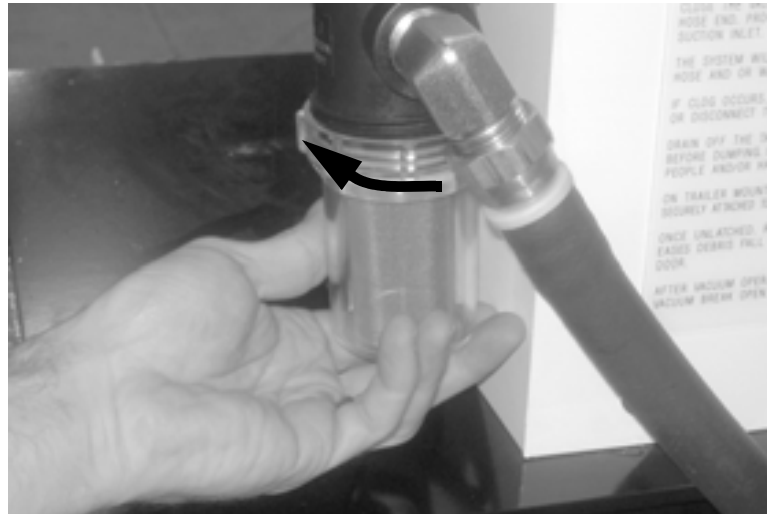
Figure 6-23. Unscrew the strainer bowl.
