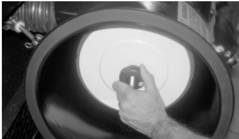
Figure 6-4. Remove the knob holding the filter in place. Be careful not to lose the washer behind the knob.
