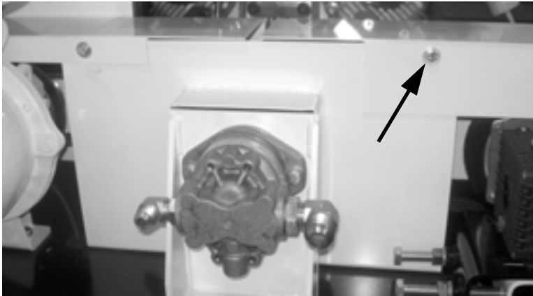
Figure 7-22. Remove the screw on the back of the sprayer pump belt cover.
