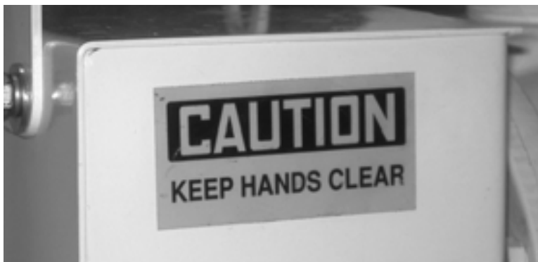
Figure 2-4. This caution label is on the belt cover toward the rear of the trailer. Keep hands away from the belt drive area while any equipment is operating or the gas engine is running. (Part no. 77-160-11.)
