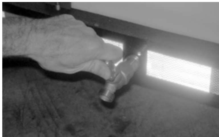
Figure 4-14. Open the drain valve on the back of the trailer to drain the water tank.
