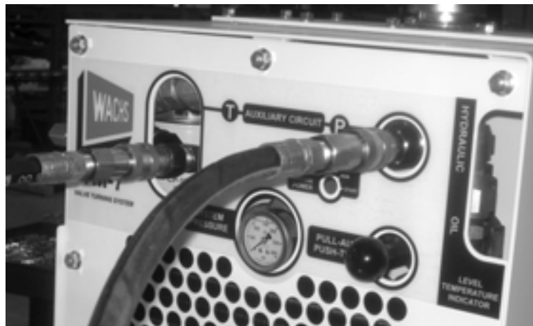
Figure 5-59. Remove the hoses from beneath the back of the trailer and connect them to the auxiliary ports on the front of the tank.
