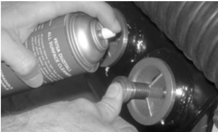
Figure 6-15. Spray lubricant on the pressure relief valves.
