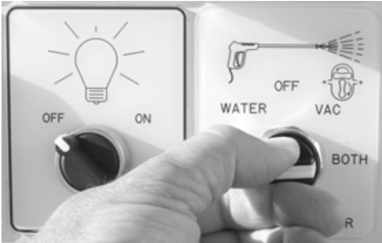
Figure 5-15. To use both the washer and vacuum, turn the Vacuum/Pressure Washer switch to the BOTH position.
