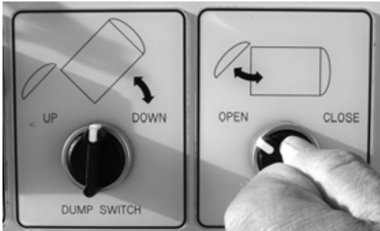
Figure 7-28. Turn the Latch Switch to the OPEN position and hold it until the latch fully opens.
