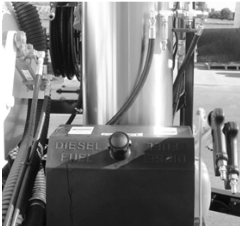
Figure 5-62. The water heater fuel tank is mounted in front of the heater.
