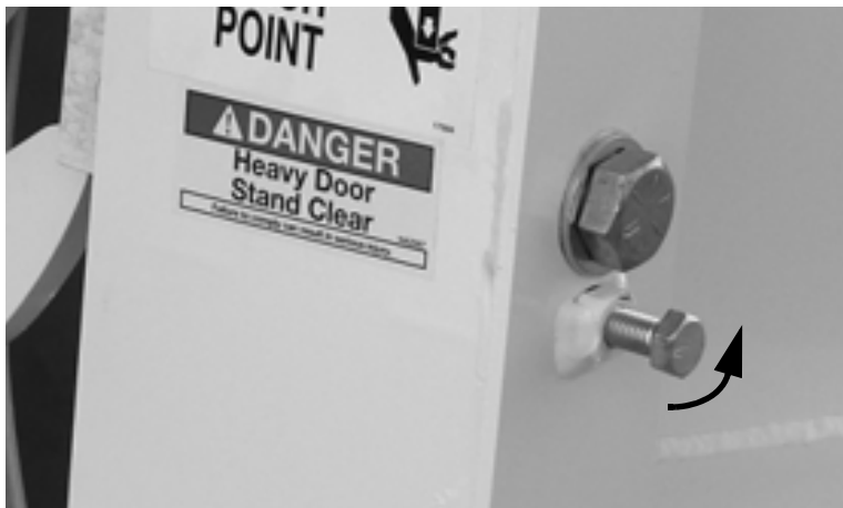
Figure 7-29. Turn the set screw counter-clockwise to loosen it.
