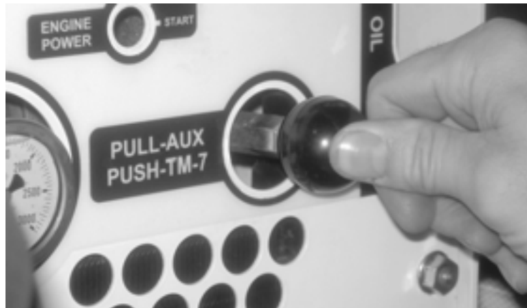
Figure 5-77. Push in the auxiliary knob to enable flow to the ERV-750.
