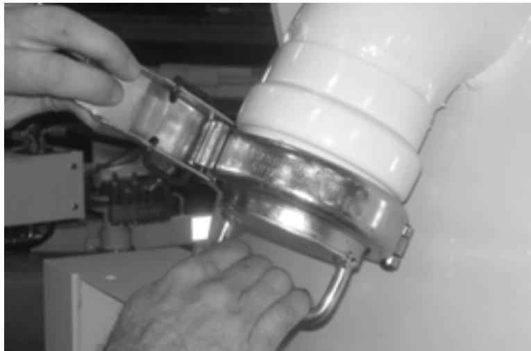
Figure 5-9. Pull the latch on the locking collar to release it and take it off the inlet port.
