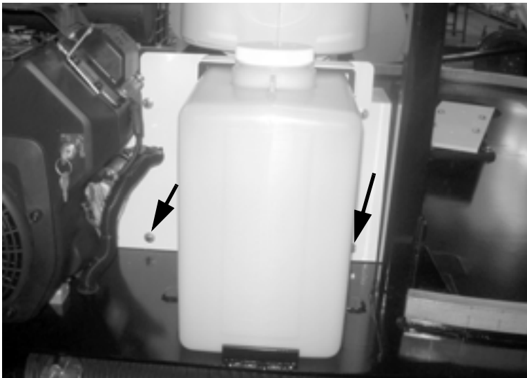
Figure 7-19. After removing the priming tank, remove the two bottom screws in the belt cover.
