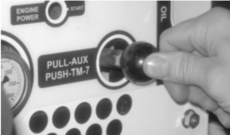
Figure 5-72. Push in the auxiliary knob to enable flow to the TM-7.
