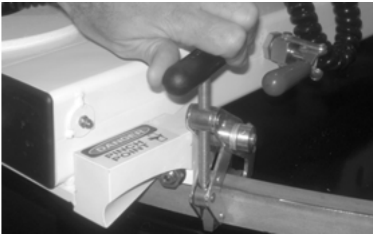
Figure 5-73. Turn the swivel clamp knob counter-clockwise to loosen the clamp. There is a clamp on each side of the TM-7.
