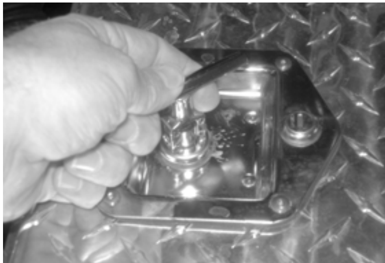
Figure 5-4. Lift the handle and turn it to open the job box.
