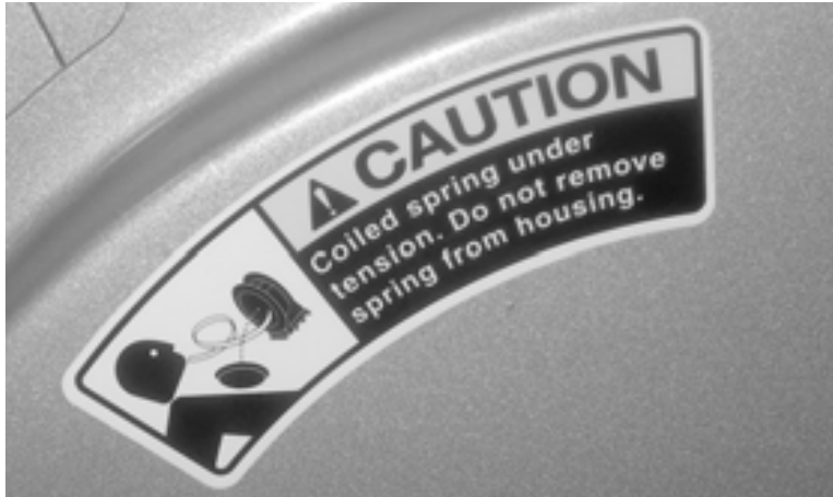
Figure 2-8. This caution label is on the hydraulic hose reel. Do not disassemble the spring from the reel. (Contact the manufacturer, Cox Reels, for replacement label.)
