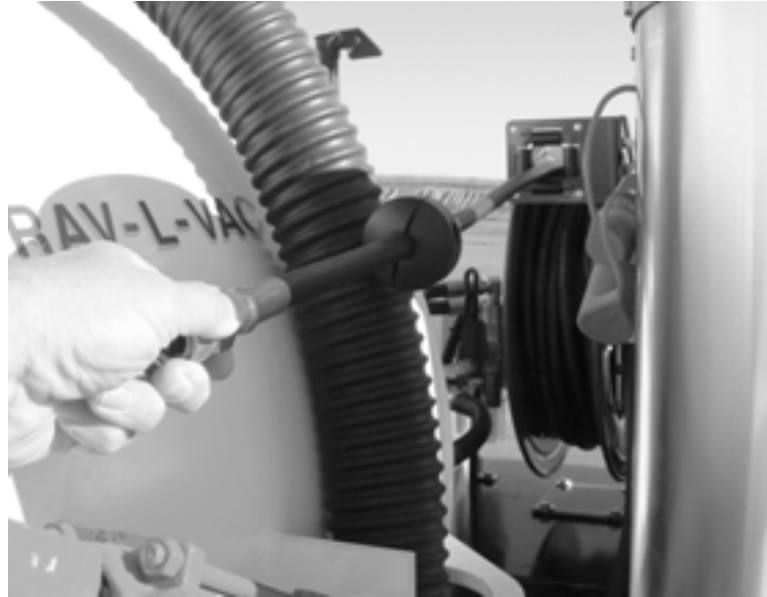
Figure 5-35. Pull the sprayer hose out of the hose reel until it reaches the work location.
