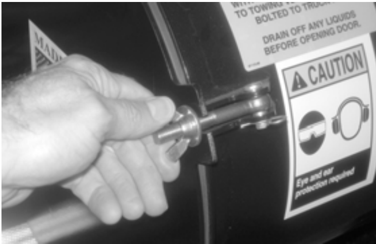
Figure 6-2. Loosen the wing nuts on the three filter canister latches far enough to swing the latches back.
