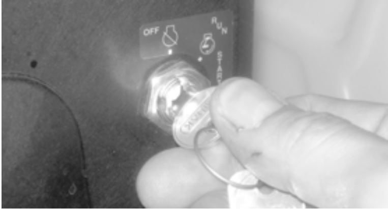
Figure 5-6. Turn the engine key to START. Release it to RUN when the engine starts.
