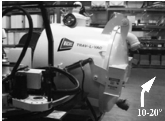
Figure 5-23. Turn the Dump Switch to the UP position and hold it just until the tank has cleared the deck and begins to tip (approximately 10° - 20°).
