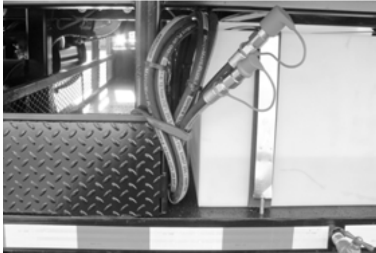
Figure 5-58. The hose connections to the hydraulic hose reel are stored under the trailer between the storage box and water tank. Remove the strap to take the hoses out and connect them.
