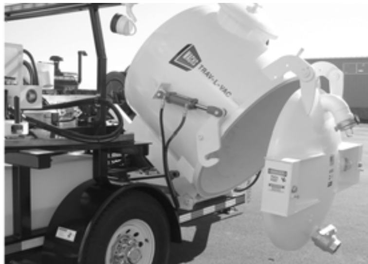
Figure 5-27. Tank in the fully tipped position.
