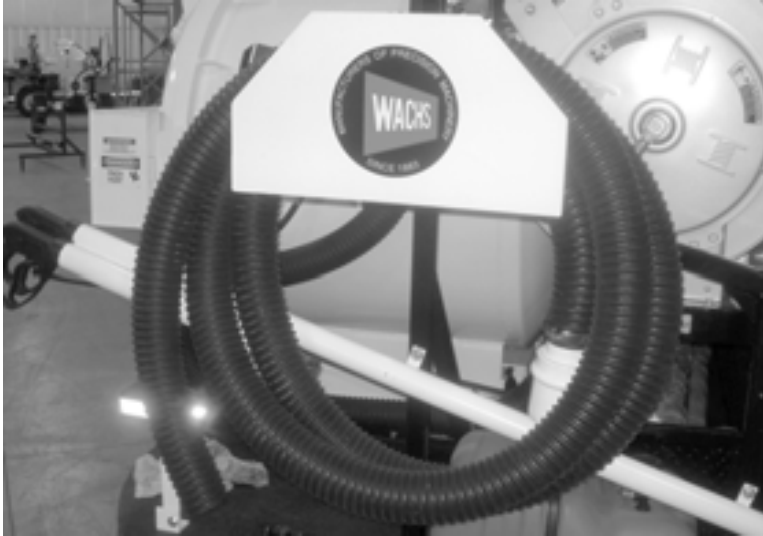
Figure 3-10. The vacuum hose is rolled up and stored on the front of the trailer.
