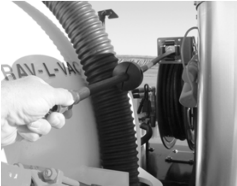
Figure 5-69. Pull enough hose out of the sprayer reel to reach the front of the water heater.
