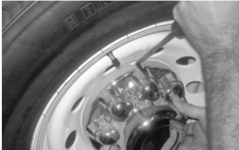
Figure 7-2. Use a standard screwdriver in the wheel cover slot to remove the cover.
