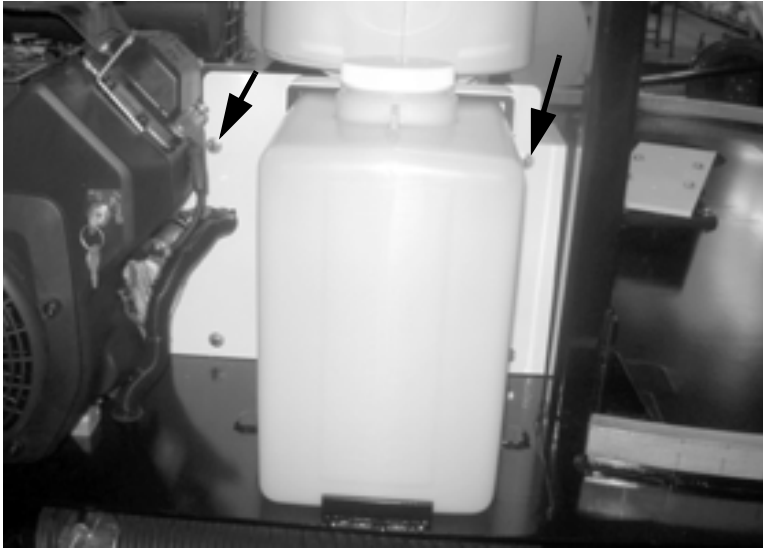
Figure 7-18. Remove the two top screws holding the priming tank bracket in place; then remove the bracket and tank.
