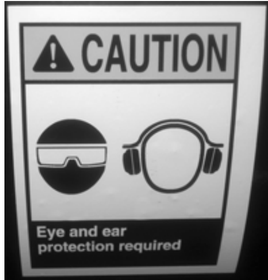
Figure 2-1. The eye and ear protection label is on the vacuum filter housing, below the control panel, and on the door of the spoils tank (3 locations). Wear protective gear when operating the vacuum system. (Part no. 77-160-05.)
