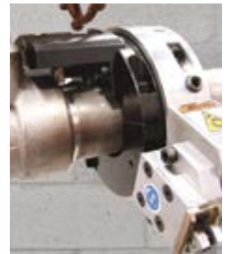
Socket Weld Removal
