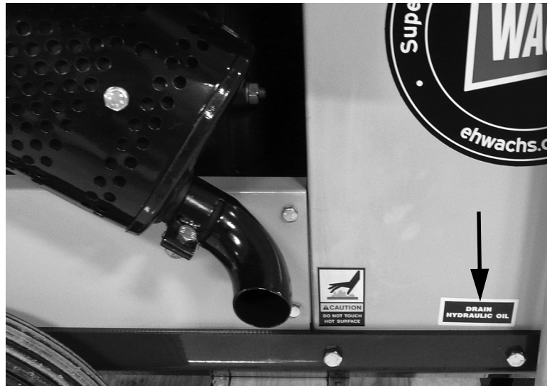
Figure 3-10. A label on the side of the HPU indicates the location of the hydraulic oil drain plug (underneath the unit).
