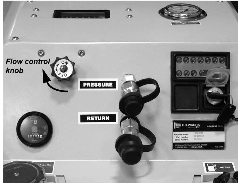
Figure 3-9. Turn the flow control in the ON direction to operate the tool. (Control panel shown without hoses attached.)
