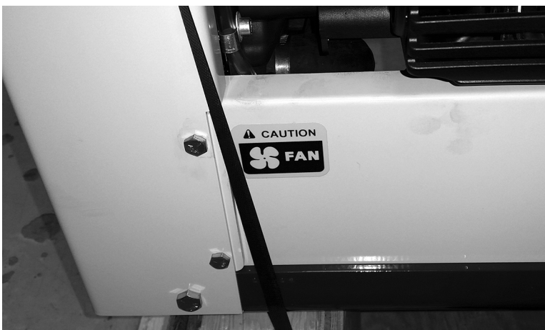
Figure 2-1. Labels on each side of the unit indicate the location of the engine fan.
