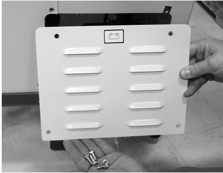
Figure 3-1. Remove the battery compartment cover.
