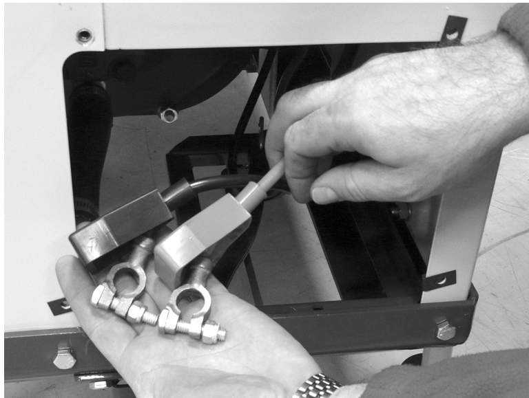
Figure 3-2. Attach the cables to the battery posts.
