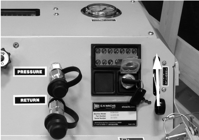
Figure 3-8. Set the throttle to the maximum speed position for operation.
