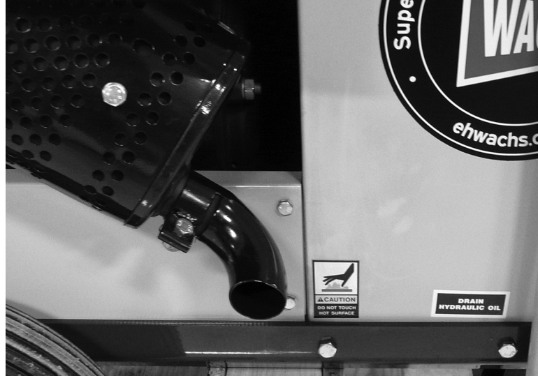
Figure 2-2. A Hot Surface label is located near the engine muffler.
