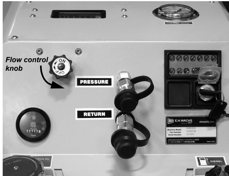
Figure 3-6. Turn the flow control all the way OFF before starting the power unit or connecting hoses.
