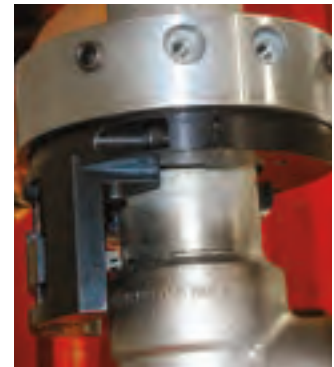
Axial Socket Weld Removal
