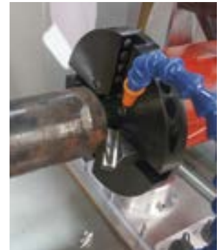
Weld Coupon Station uses coolant for extended tool life
