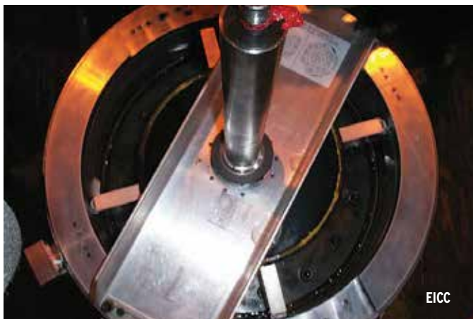
Wachs EICC system provides a fast and reliable method of cutting casings externally above the wellhead and internally below it.
