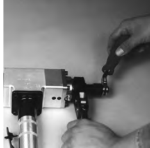
2. Remove draw bar using the clamp ratchet.
