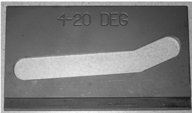
Figure 1-4. A 4-20 degree compound beveling template is provided with the single-point tool slide.\
