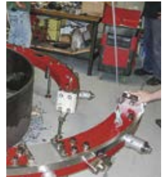
LDSF splits into quadrants for setup, transport & storage
