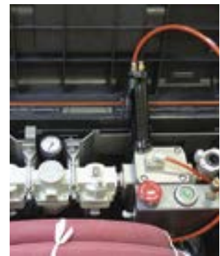
Ergonomic fingertip control with safety stop button
