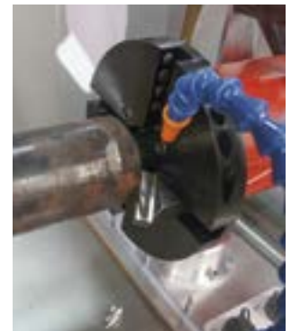
Weld Coupon Station uses coolant for extended tool life
