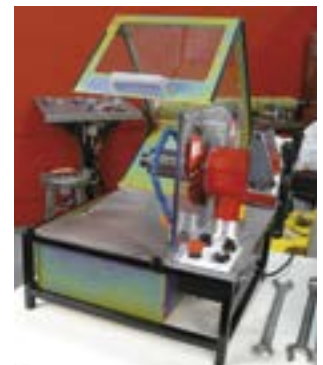
The heart of the Weld Coupon Station is the Wachs SDB 206 Beveler
