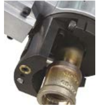
Axial tool slide accessory for socket weld removal
