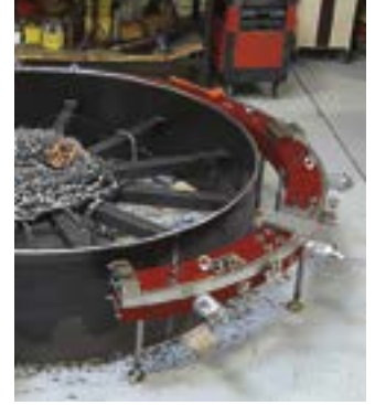
Four standard LDSF sizes cover 60-120in (DN1500-3000)
