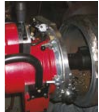
Self-centering standard mandrel
