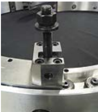
Aluminum stationary frame with steel rotating ring
