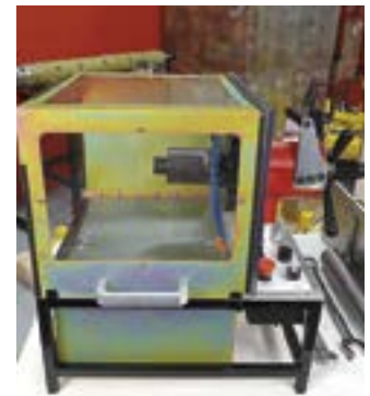
Weld Coupon Station
