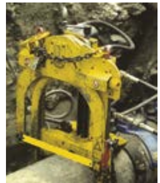
Elliptical cutting action, long blade life
