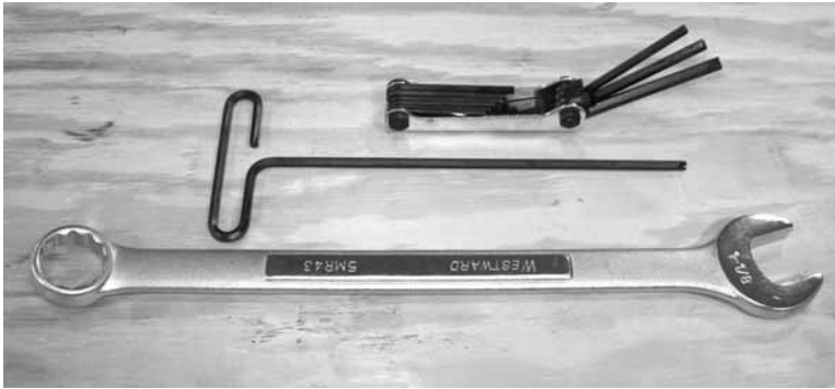
Figure 1-3. A set of hand tools is provided. The hex cluster is for maintenance, the 3/16" t-handle hex wrench is to install tooling in the rotating head, and the 1-1/8" combination wrench turns the drawbar nut.
