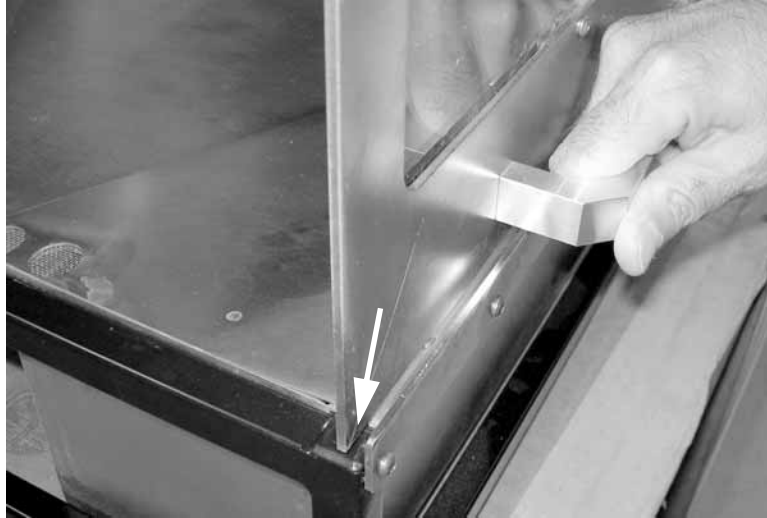
Figure 3-13. Make sure the cover rests inside the lip of the base.
