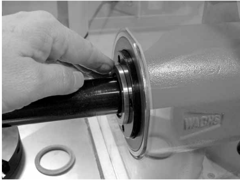
Figure 4-12. Make sure the mandrel bushing is flush with the main shaft.
