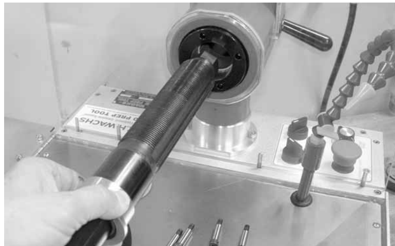
Figure 4-9. Re-insert the mandrel into the front of the machine.
