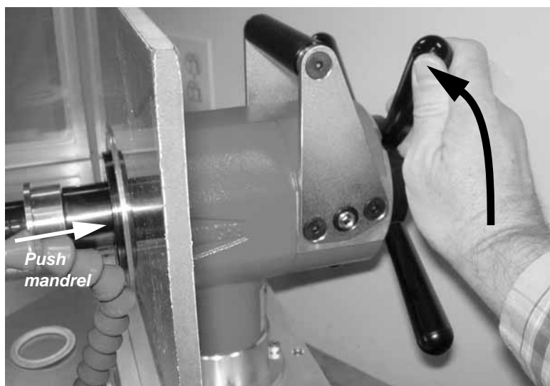
Figure 4-10. Turn the feed handle clockwise (viewed from the back of the machine) to thread the mandrel back into the feed nut. Push the mandrel in while you start the threads.
