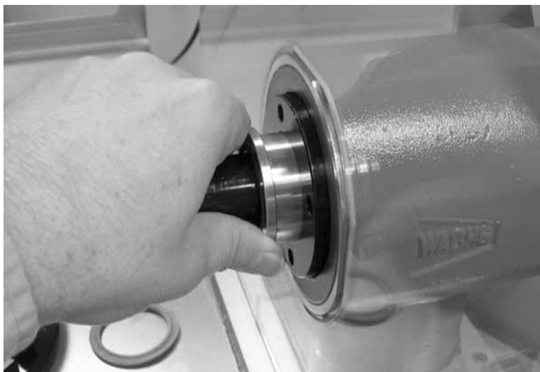
Figure 4-11. Make sure the mandrel bushing goes into the main shaft.
