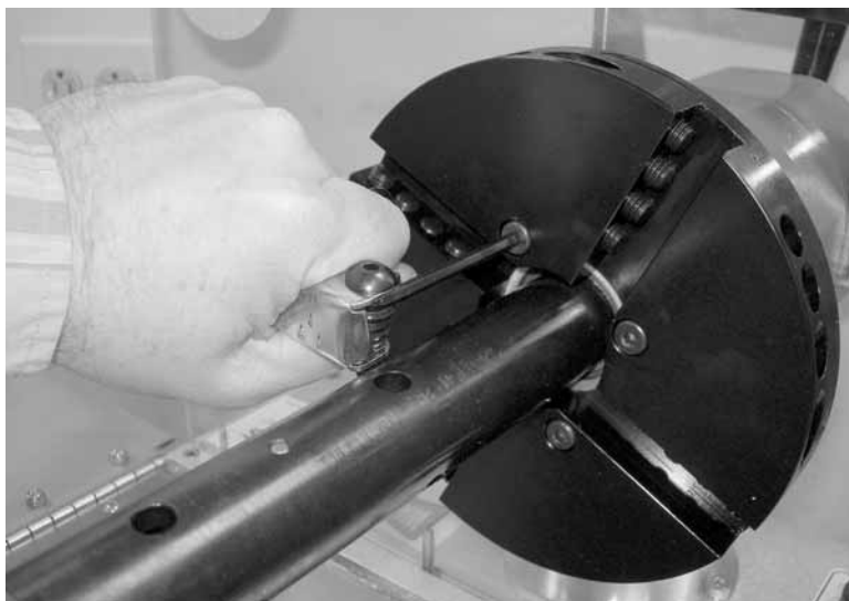
Figure 4-15. Snug all 4 screws, then tighten them securely.
