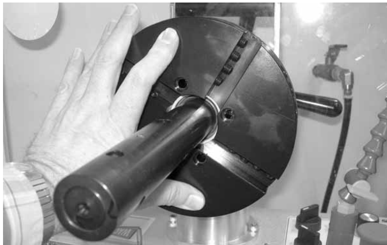
Figure 4-13. Put the tool head back onto the mandrel and line up the holes with the holes in the main shaft.
