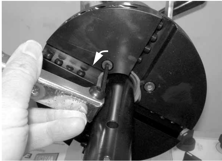
Figure 4-4. Loosen the 4 screws holding the tool head to the main shaft.
