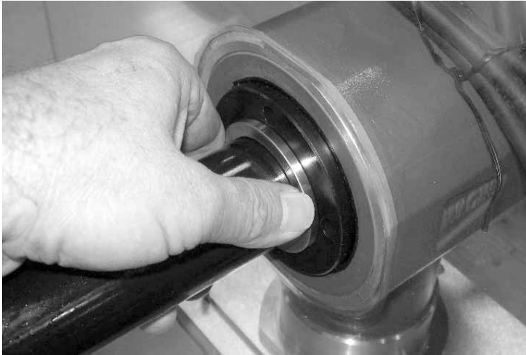
Figure 4-18. Push the bushing flush against the front surface of the main shaft.
