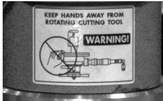
Figure 2-1. The Warning label is on the SDB 206 machine body.
