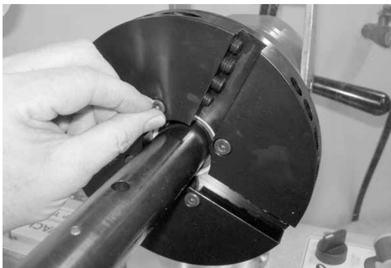
Figure 4-14. Insert the screws through the tool head into the main shaft.
