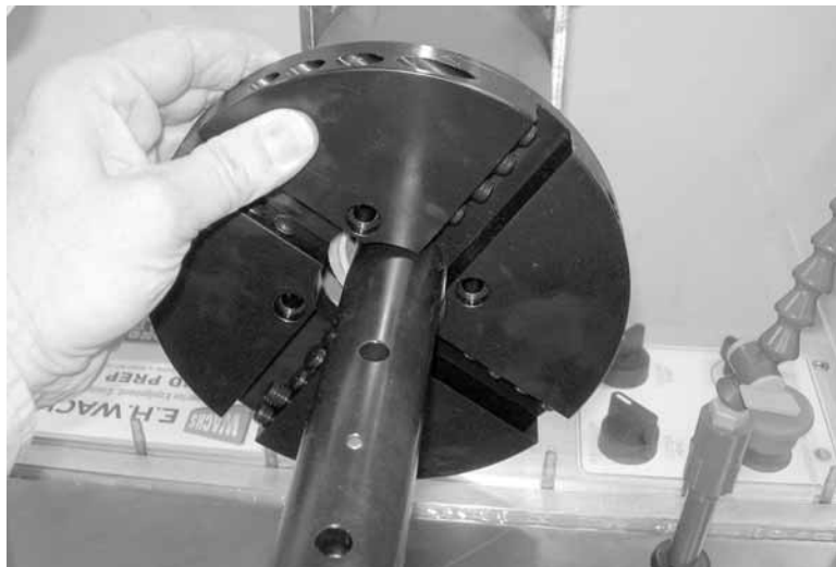
Figure 4-5. Remove the tool head from the mandrel.
