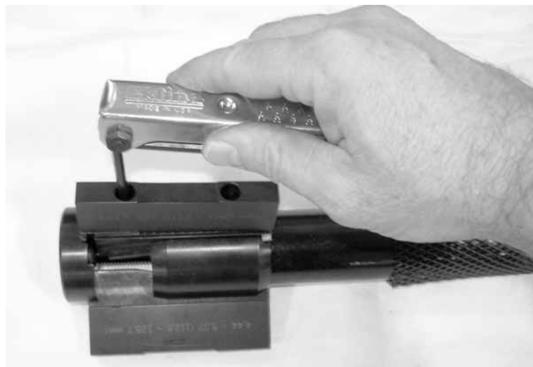
Figure 3-11. Attach the clamp legs to the mandrel. You can do this before or after installing the mandrel in the machine.
