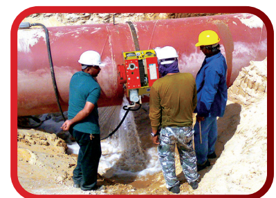
Trav-L-Cutter SD can operate on varying pipe diameters by adding additional chain sections
