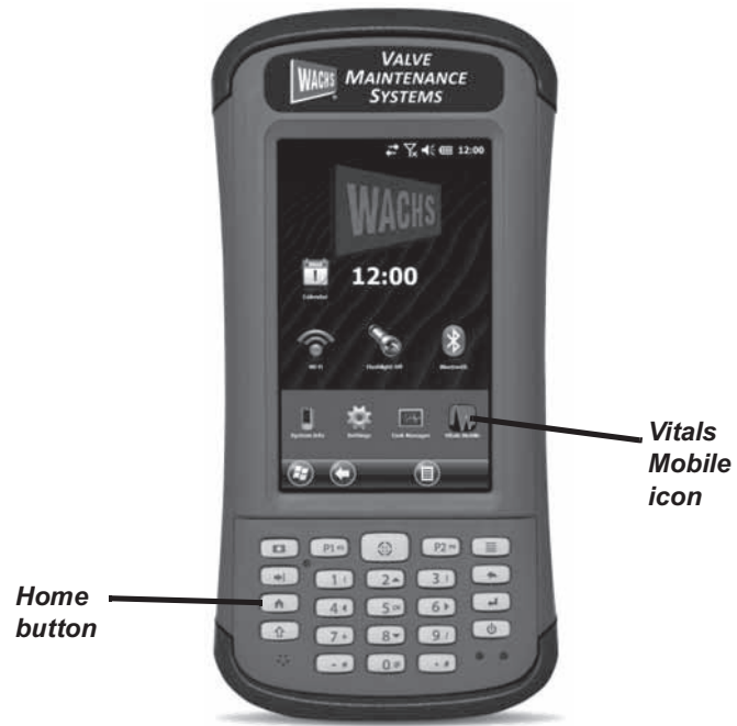
Figure 5-6. HC-100 home screen. Press the Home button on the keypad at any time to return to the home screen.
