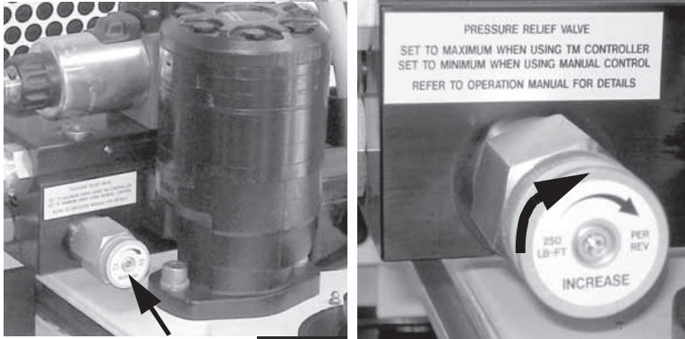
Figure 5-4. Turn the pressure relief knob all the way clockwise for maximum pressure when operating the TM-7 using the Vitals HC-100 controller.
