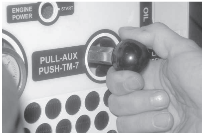
Figure 5-25. Pull out the port selector knob to operate the auxiliary circuit.
