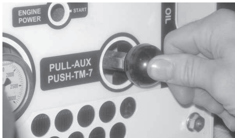
Figure 5-26. Push the port selector knob back in when you are finished using the auxiliary circuit.
