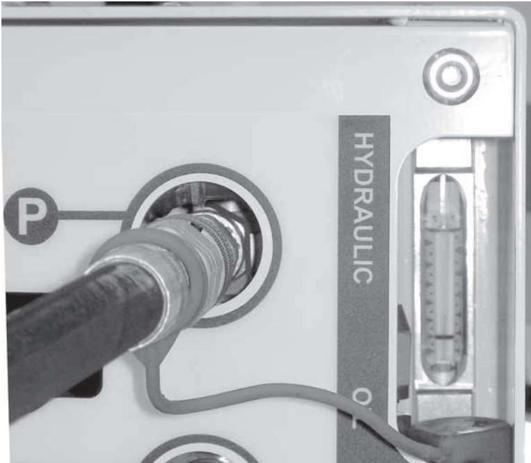
Figure 6-3. Check the oil level in the hydraulic oil gauge. The gauge also indicates temperature.
