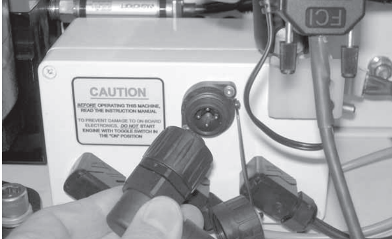
Figure 3-4. To connect the controller cable to the TM-7, unscrew the connector cap and then screw on the cable connector.
