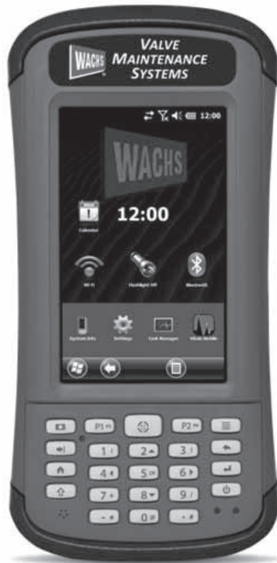
Figure 3-1. The Vitals HC-100 controller is used to operate the TM-7 and other E.H. Wachs valve operators. The controller stores valve exercising data for valve logging and analysis using the Vitals Desktop software program.
