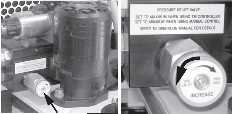
Figure 5-20. Turn the pressure relief knob all the way counter-clockwise to start at minimum pressure when operating the TM-7 using the manual controls.
