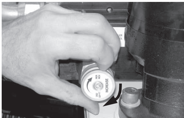
Figure 5-23. To increase the torque, turn the pressure knob clockwise. Each turn increases the torque by approximately 250 lb-ft. Do not increase the pressure more than one turn at a time.
