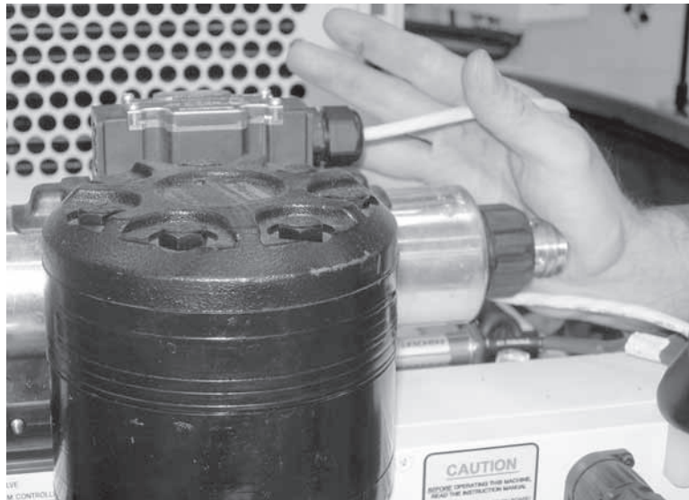
Figure 5-22. Press in the right flow control to turn the valve clockwise .
