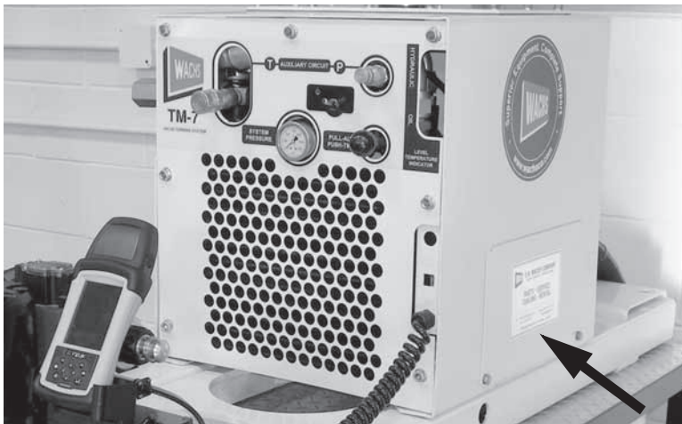
Figure 5-28. Remove the battery cover on the side of the TM-7 enclosure.
