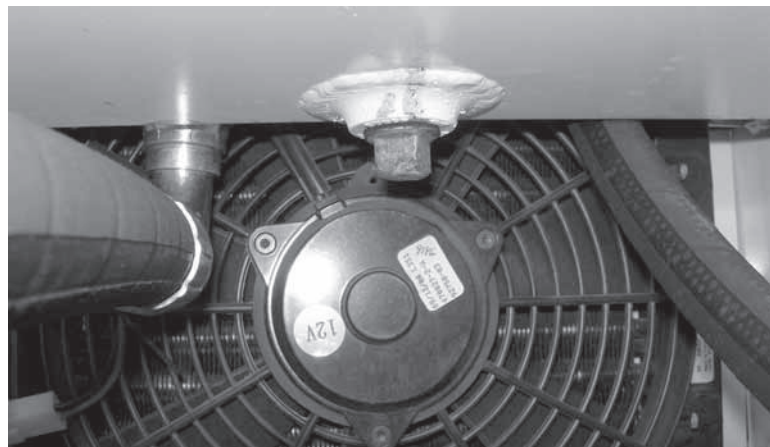
Figure 6-5. The hydraulic reservoir drain plug is accessible through the back of the TM-7 enclosure.
