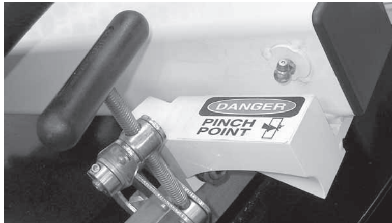
Figure 2-2. Keep hands clear of the swivel rail when positioning the TM-7.
