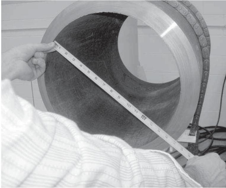
Figure 5-1. Measure the I.D. of the pipe to determine which leg set will be required.
