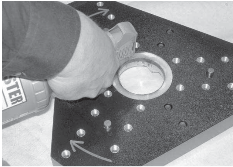
Figure 6-4. Apply oil to the felt wiper in the rotating head.
