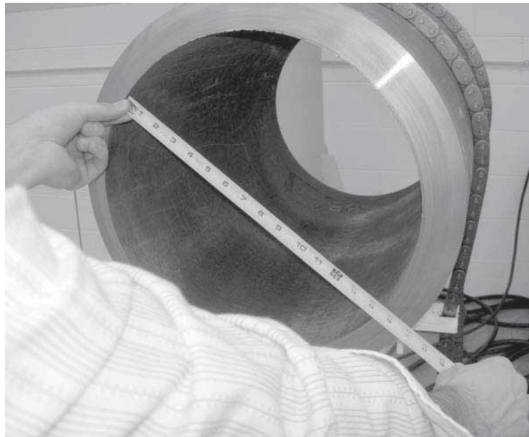
Figure 5-8. Measure the I.D. of the pipe to determine which leg set will be required.
