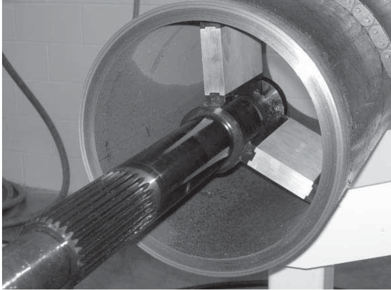
Figure 5-5. Insert the clamping legs into the pipe.
