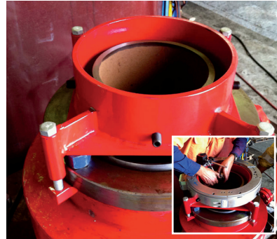
Figure 3 - Adaptors available for most manufactured wellheads
