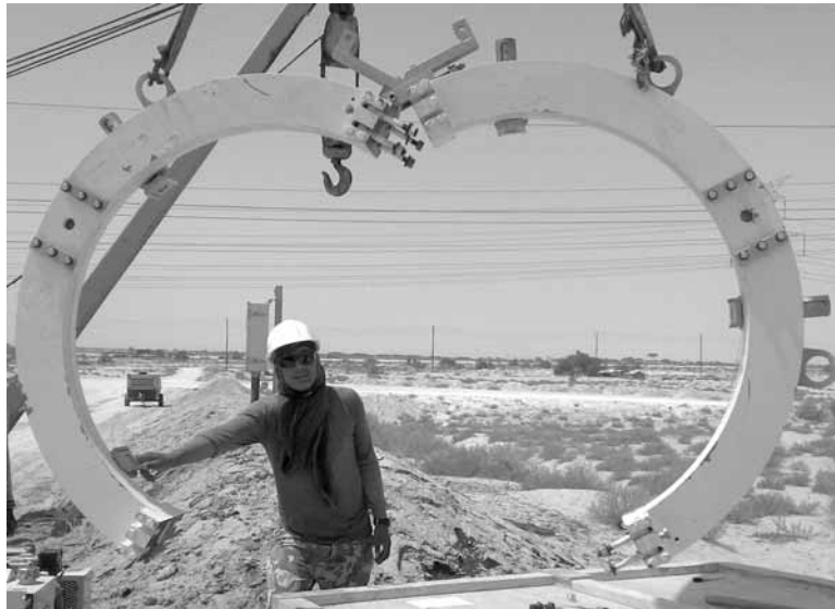
Figure 3-1. The photo shows the HDSF opened for mounting on inline pipe.
