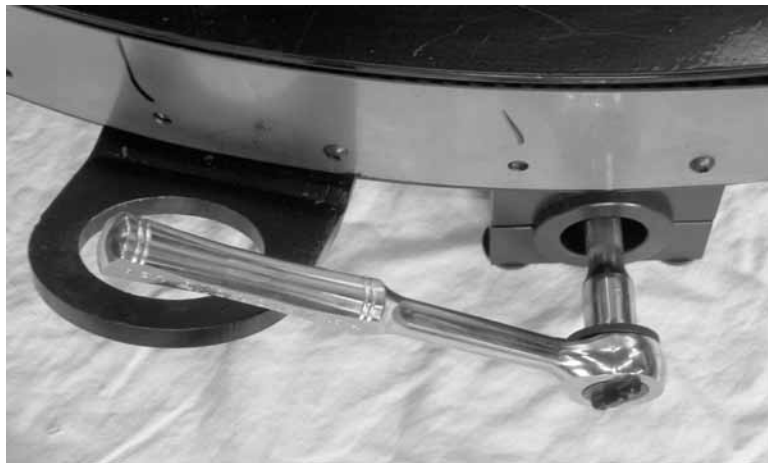
Figure 5-9. Tighten the clamping pads using a 1-1/8" socket inserted through the back of the clamping leg.
