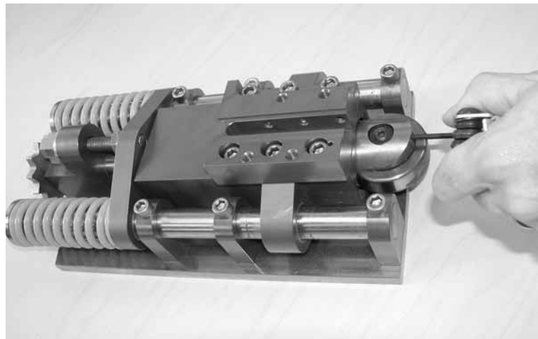
Figure 7-6. Remove the set screw holding the tracking wheel shaft.
