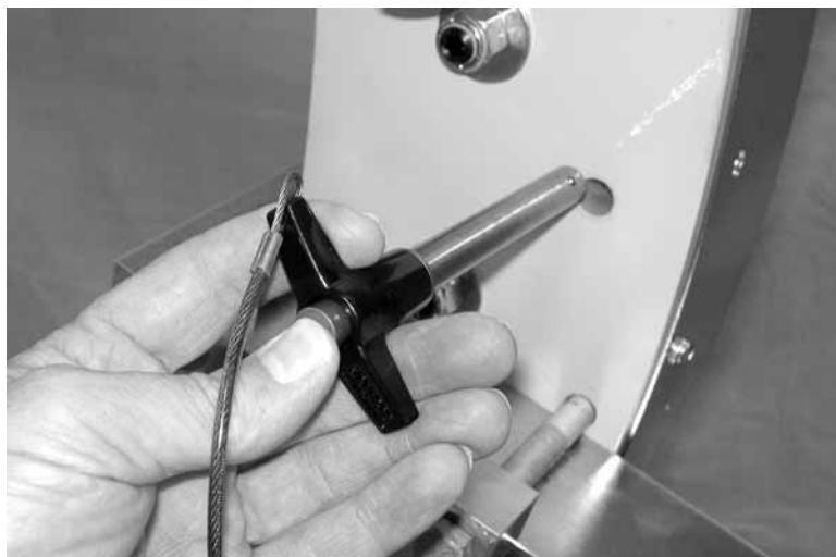
Figure 7-2. Insert the frame locking pins to lock the stationary and rotating rings together.
