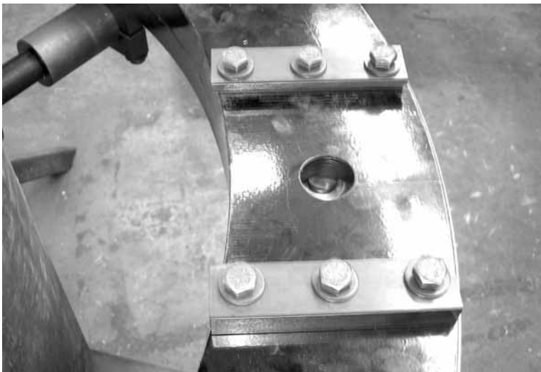
Figure 5-21. Install the slide mounting blocks on the rotating ring. Leave the mounting bolts loose.
