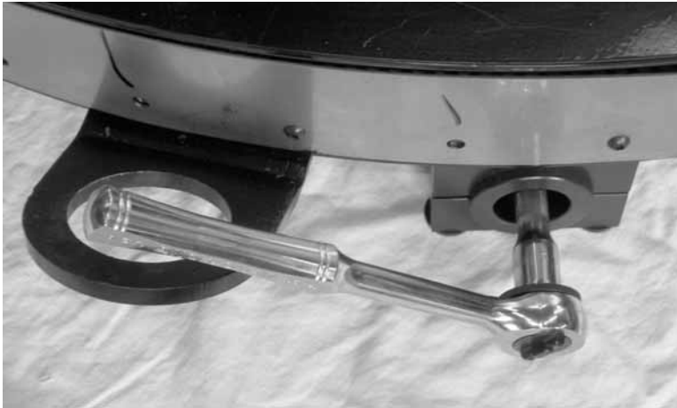
Figure 5-6. Use a 1-1/8" socket inserted through the back of the clamping leg to screw the clamping pads all the way back.
