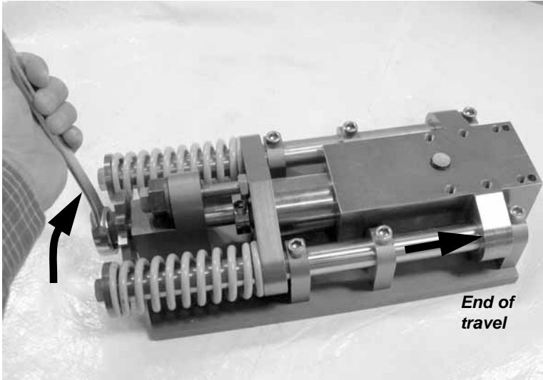
Figure 7-11. Turn the feed nut counter-clockwise to advance the slide to the end of travel.
