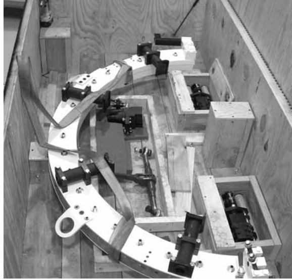
Figure 4-6. Put the first half of the ring into the crate as shown. The ends of the ring should rest on the support blocks in the corners.
