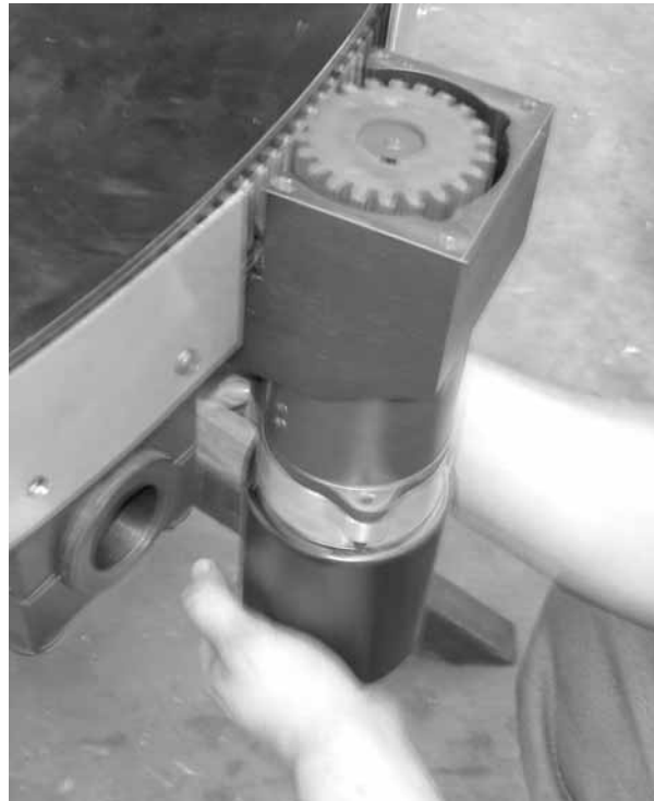
Figure 5-19. Install the air motor on the frame and tighten the two bolts (underneath) that secure it.
