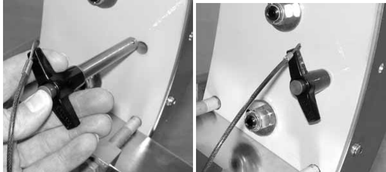
Figure 5-2. Insert both frame locking pins through the stationary ring and rotating ring. Press the button on the handle of the pin to insert or remove it.
