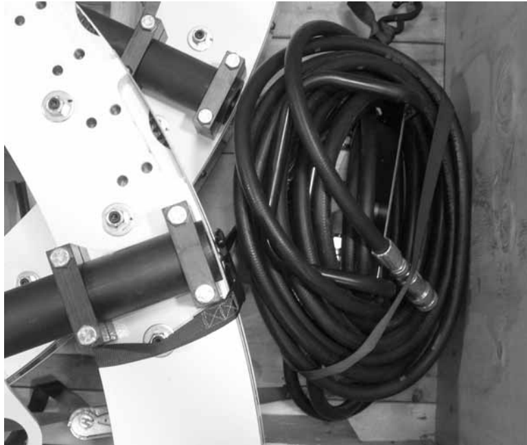
Figure 4-8. Put the flow control assembly along the side of the case.
