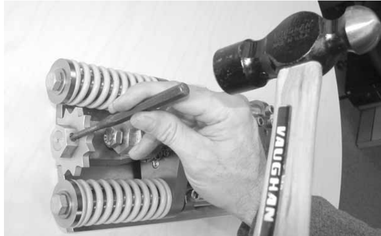
Figure 7-17. Use a punch to remove the roll pin holding the starwheel in place, then pull the starwheel off the feed shaft.
