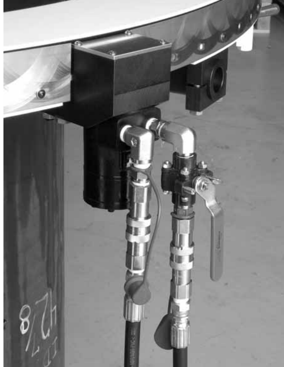
Figure 5-14. Install the hydraulic motor on the frame at the mounting location.
