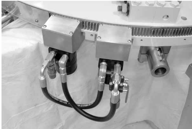
Figure 3-8. The photo shows the HDSF with dual motor drive configuration.
