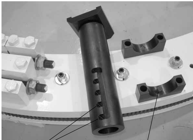
Figure 5-7. The position notches in the leg fit onto the pin in the outside clamping block. The notches are 1" (25 mm) apart.
