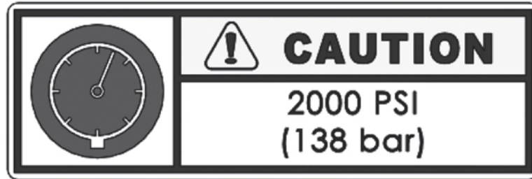
Figure 2-5. The hydraulic pressure label is attached to the SDB 206/FF 313 hydraulic drive. Do not operate the equipment with greater than 2000 psi (138 bar) hydraulic pressure. (Part no. 90-402-01.)
