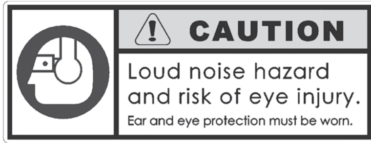
Figure 2-2. The ear and eye protection label is attached to the air and electric drives of the SDB 206/FF 313. Always wear ear and eye protection when operating the equipment. (Part no. 90-401-03.)
