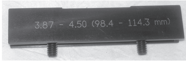
Figure 1-6. The pipe I.D. diameter range is stamped on each leg set. Each leg has two captivated mounting screws that attach the leg to the chuck leg on the mandrel.
