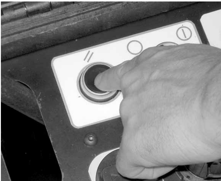
Figure 5-45. The Reset button resets the ACM after a loss of pressure or an emergency stop.
