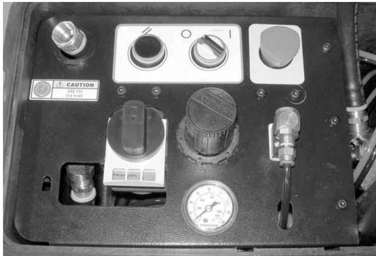
Figure 5-39. The ACM controls should be in the pre-operation state, as shown, before connecting the air lines.
