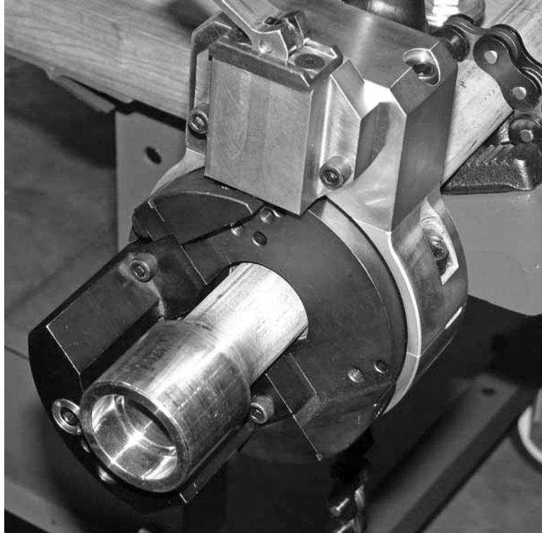
Figure 5-31. The photo shows the axial socket weld slide in position for socket weld removal.
