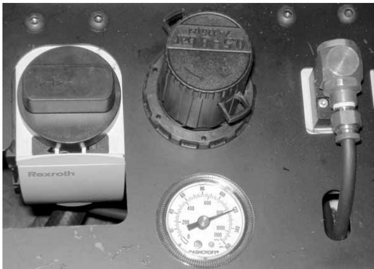
Figure 5-49. Without pulling the pressure knob, you can turn it to expose the lock tabs. Put a lock through the tab to prevent the pressure from being adjusted.
