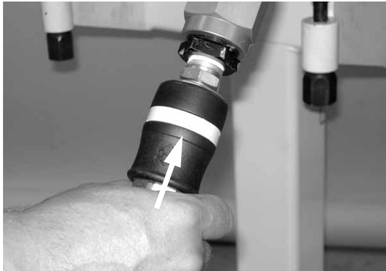
Figure 5-50. Push the air line disconnect onto the air drive fitting until it locks in place.
