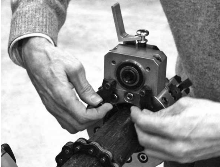
Figure 5-20. Pivot the clamps downward to attach the drive.
