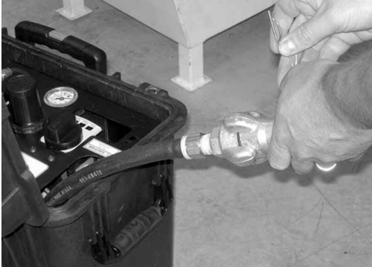
Figure 5-40. Connect the line from the air source to the input connector on the ACM.
