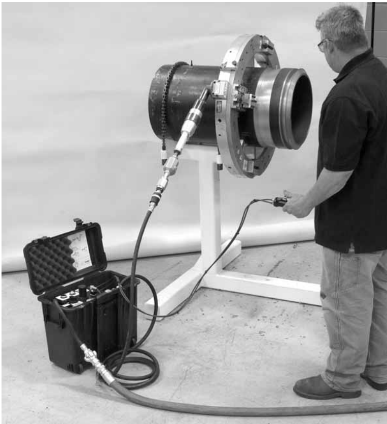
Figure 5-38. Position the ACM at a convenient distance from the split frame machine.
