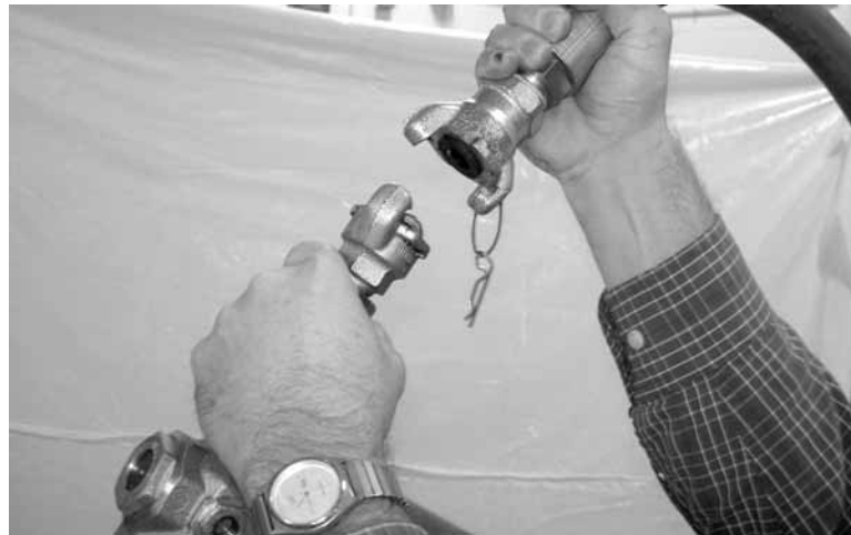
Figure 2-4. Disconnect pneumatic power by removing the air line from the pneumatic drive.
