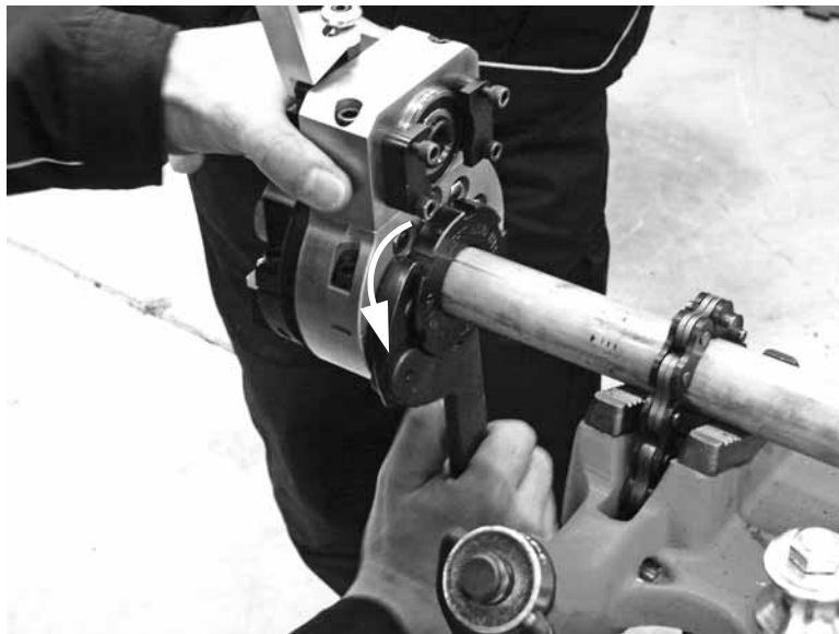
Figure 5-19. Turn the collet nut counter-clockwise to tighten it.
