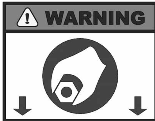
Figure 2-5. This label is on the pinion housing. The motor clamps must be secure to operate the SDSF safely.
