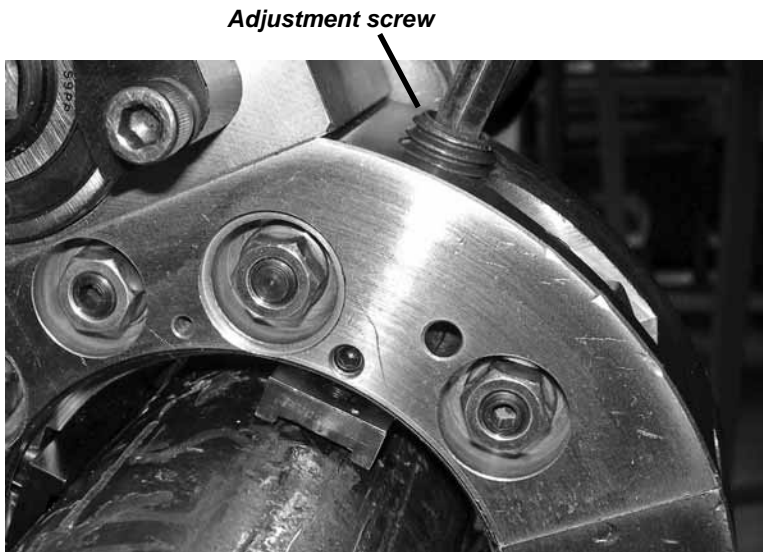
Figure 3-5. Turn the adjustment screw to tighten or loosen the clamp foot.
