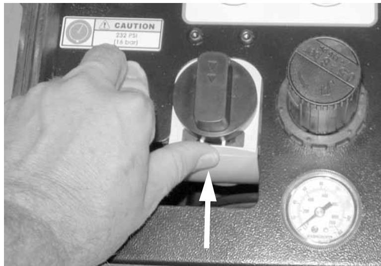
Figure 5-43. Press in the lock-out tab to enable the ON/OFF valve.
