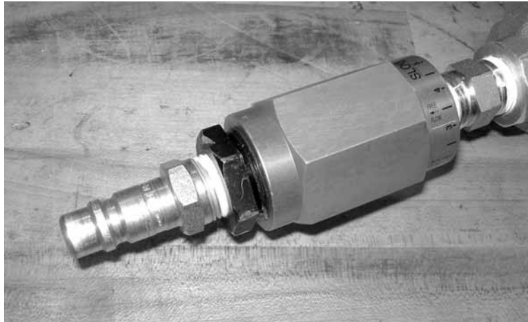
Figure 5-53. Install the supplied nipple onto the air motor for use with the ACM.
