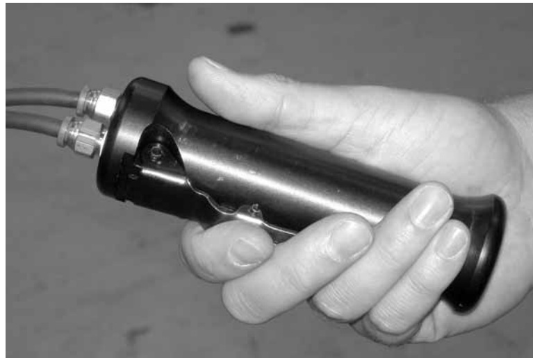
Figure 5-47. Squeeze the trigger on the handheld pendant to operate the machine.
