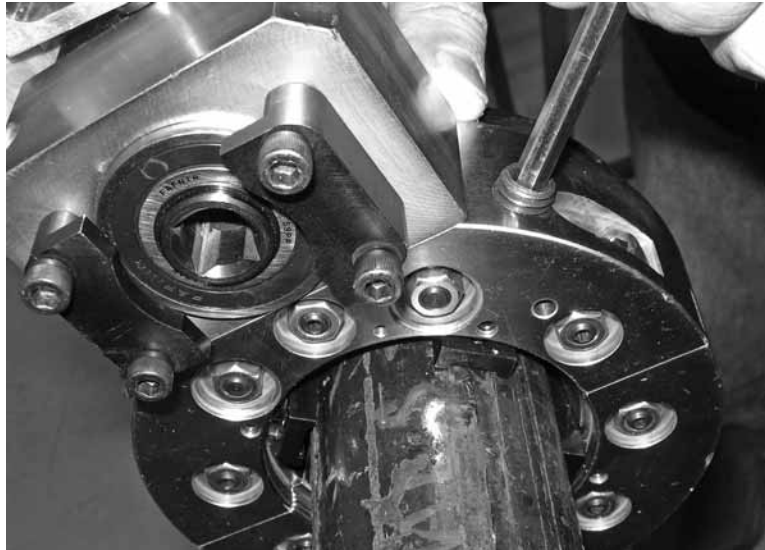
Figure 5-12. Tighten the clamp feet as indicated.
