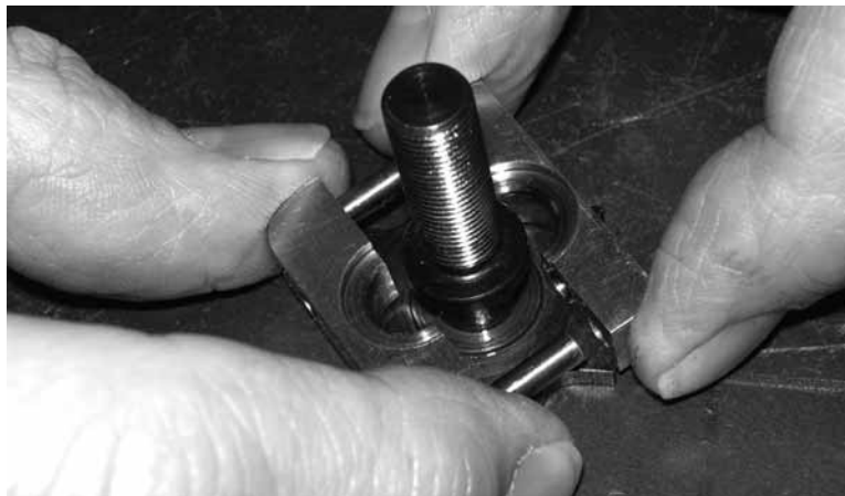
Figure 7-5. Align the bushing pins by hand, and then tap the bushing halves flush with a mallet.
