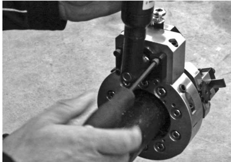
Figure 5-21. Tighten the motor clamp screws to secure the motor in place.
