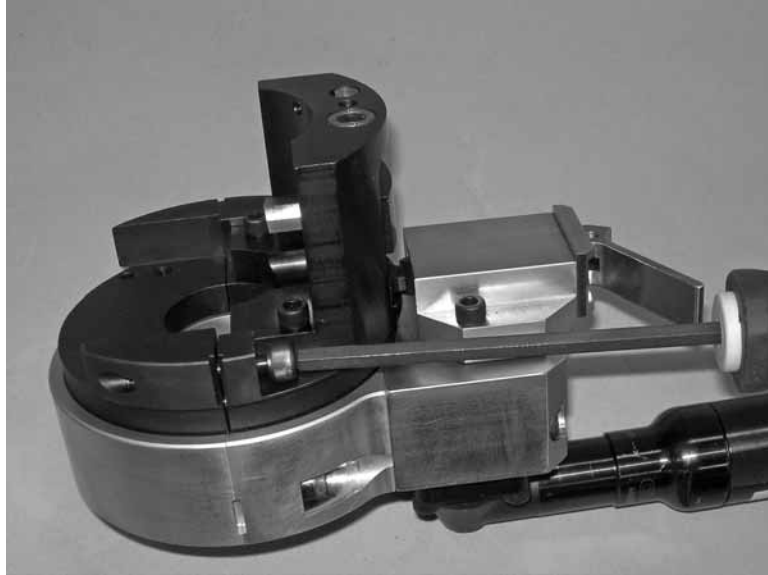
Figure 5-15. Loosen the frame locking screws in both the rotating and stationary rings.
