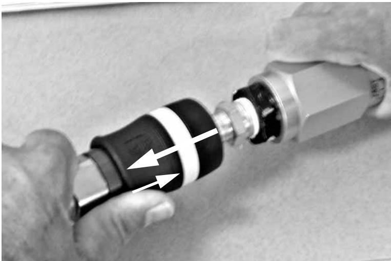
Figure 5-52. Push the collar forward and pull the disconnect to remove it from the fitting.
