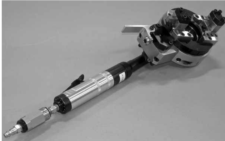
Figure 3-14. The pneumatic drive (80-4004-00) can be used to power any size SDSF.
