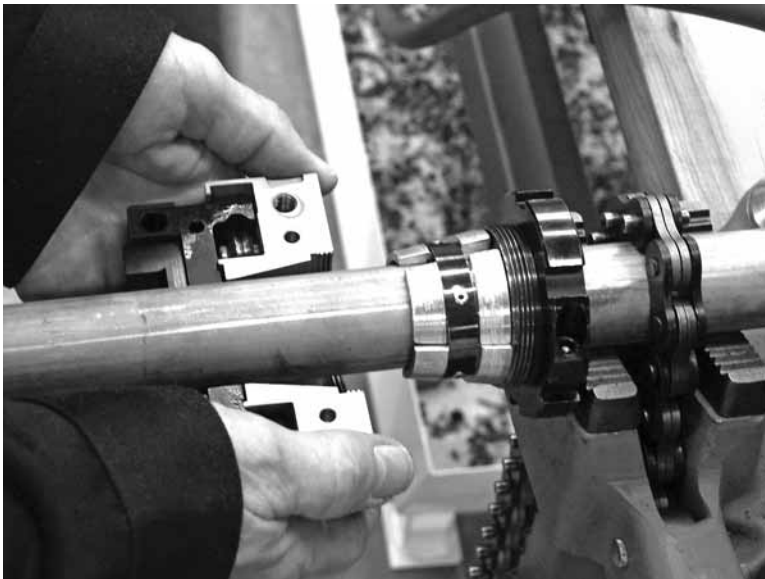
Figure 5-17. The collet mounting is self-centering when assembled properly.
