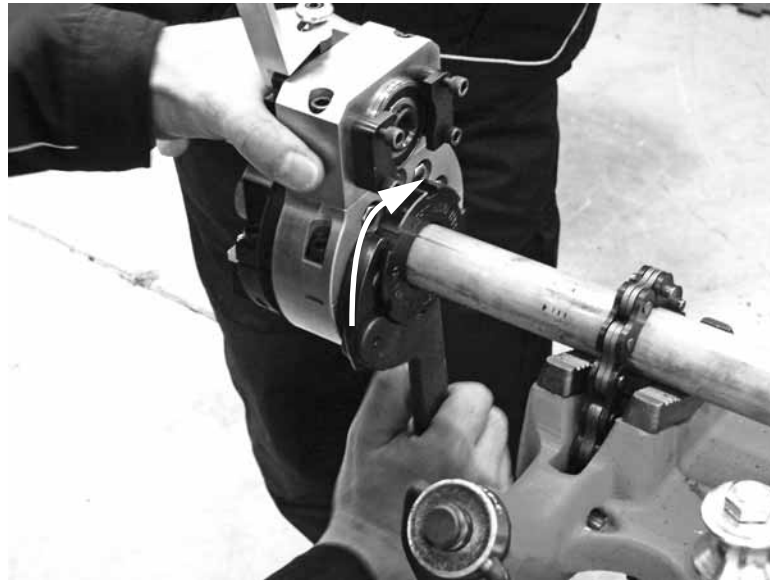
Figure 5-35. Turn the collet nut clockwise to loosen it.
