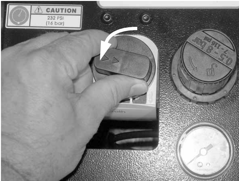
Figure 5-44. Turn the ON/OFF valve counter-clockwise to the ON position (shown in OFF position).
