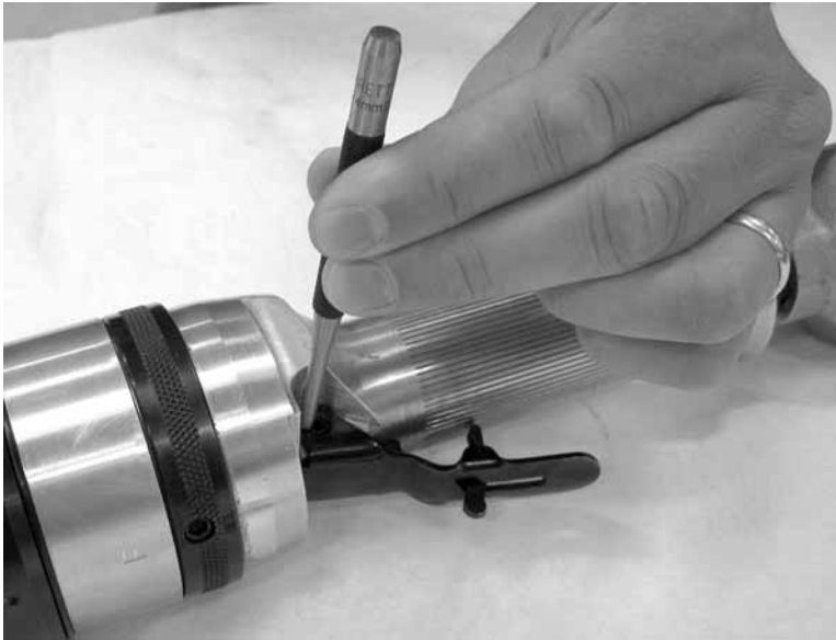
Figure 5-54. Use a punch to drive out the pin holding the air trigger.
