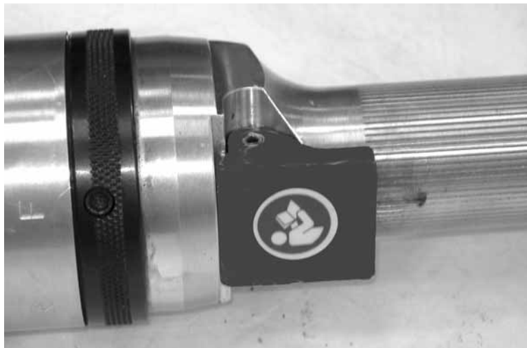
Figure 5-57. The photo shows the correct installation of the open throttle plate.
