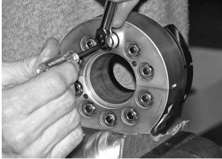
Figure 6-8. Tightening the topmost bearing centers all of the bearings.
