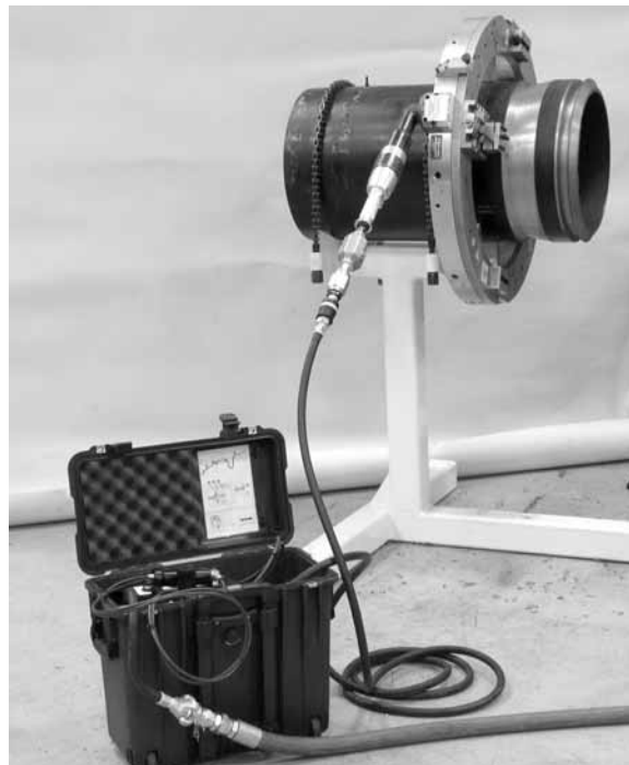
Figure 5-41. Route the hoses so they do not touch moving parts of the split frame.
