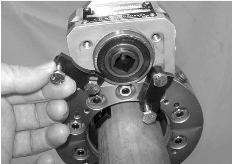
Figure 5-23. Loosen the clamp screws and swing the clamps downward to provide clearance for attaching the electric drive.
