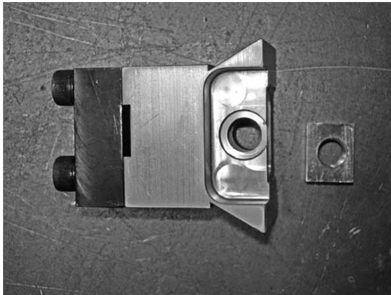
Figure 7-2. Replace the old feed nut in the slide.
