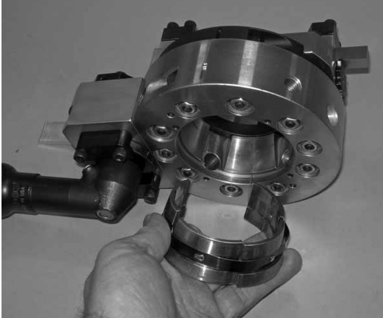
Figure 5-13. Remove the collet from the SDSF before mounting the machine on the pipe.
