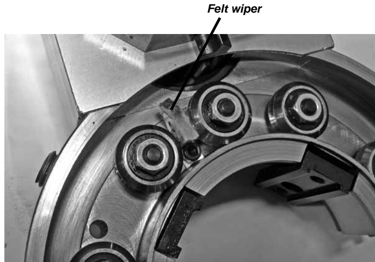
Figure 4-1. Oil the felt wiper after every use of the machine.
