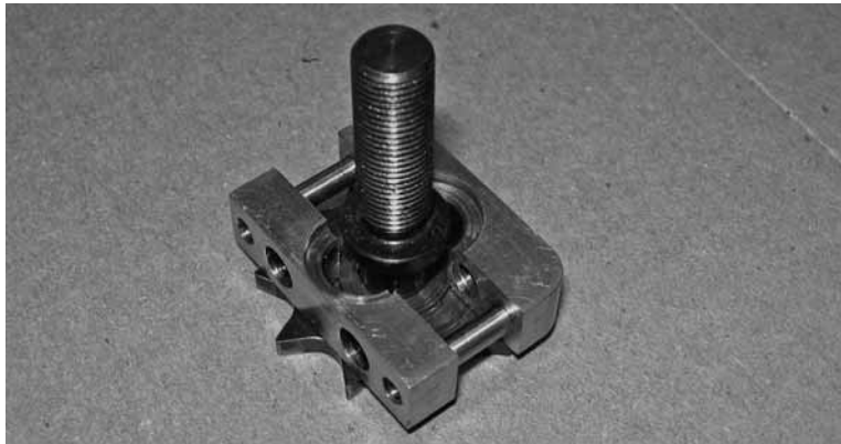
Figure 7-4. Use a mallet to separate the feed bushing as shown.
