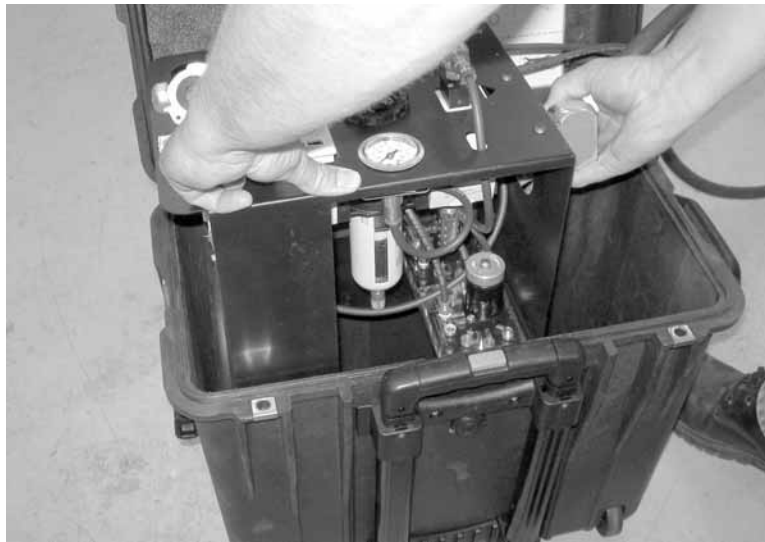
Figure 6-12. Lift the control panel out of the case for service or to drain out accumulated water.
