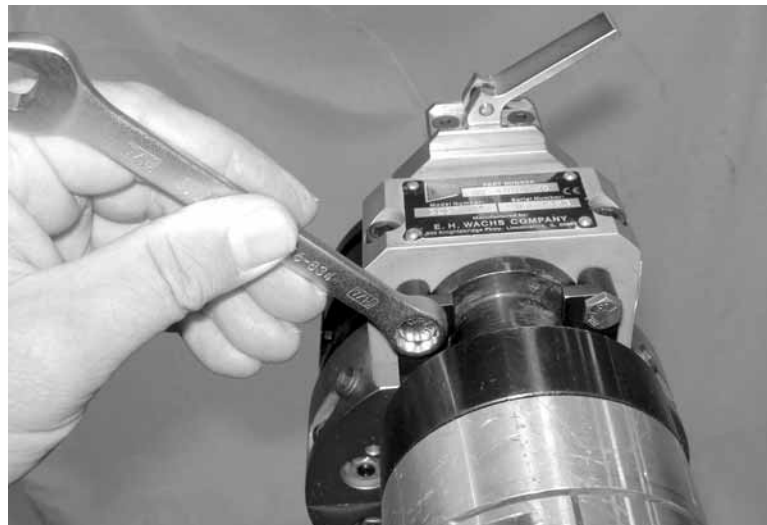
Figure 5-25. Put the clamps back in place over the flange and tighten the clamp screws with the supplied 7/16" combination wrench.
