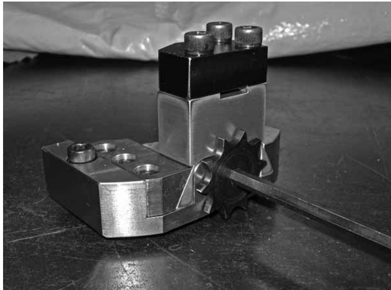
Figure 7-1. Use a hex wrench to turn the starwheel clockwise to remove the male tool slide.
