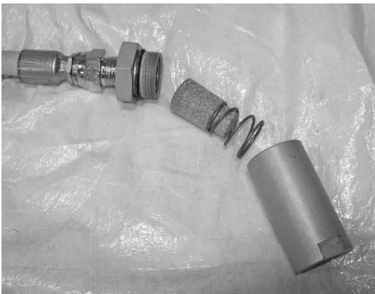
Figure 6-4. Inspect the air filter weekly. Replace as needed.
